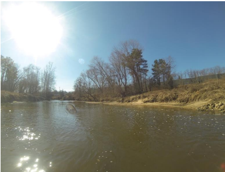
Figure 2. Hoop net deployed in new location in Cameron Run. The hedging is angled downstream in order to funnel up-migrating herring into the opening of the net.
