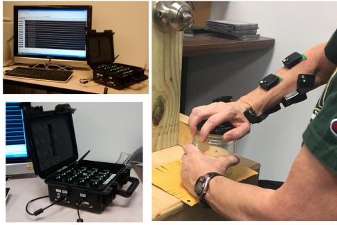
Figure 2.1: Trigno kit used for data collection (left, top and bottom) and a subject (right) performing a jar lid turn with ten sensors attached to the action arm[1]
