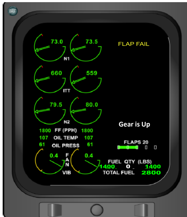
Figure 3.2: Flap failure notification.
