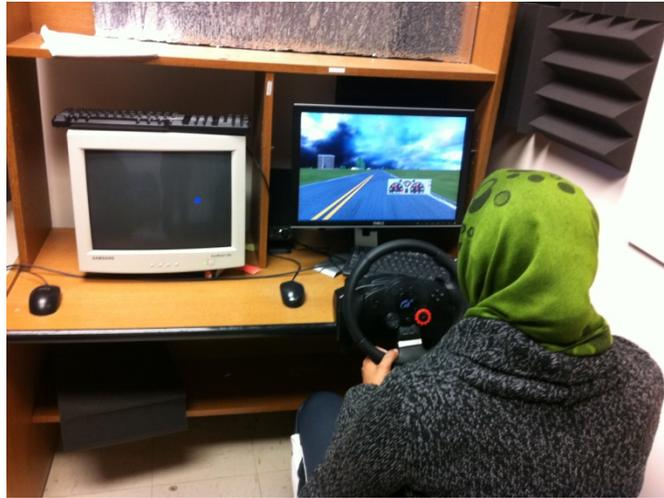
*Figure 3.* Experiment set-up with PDT task placed to the left of driving display.
