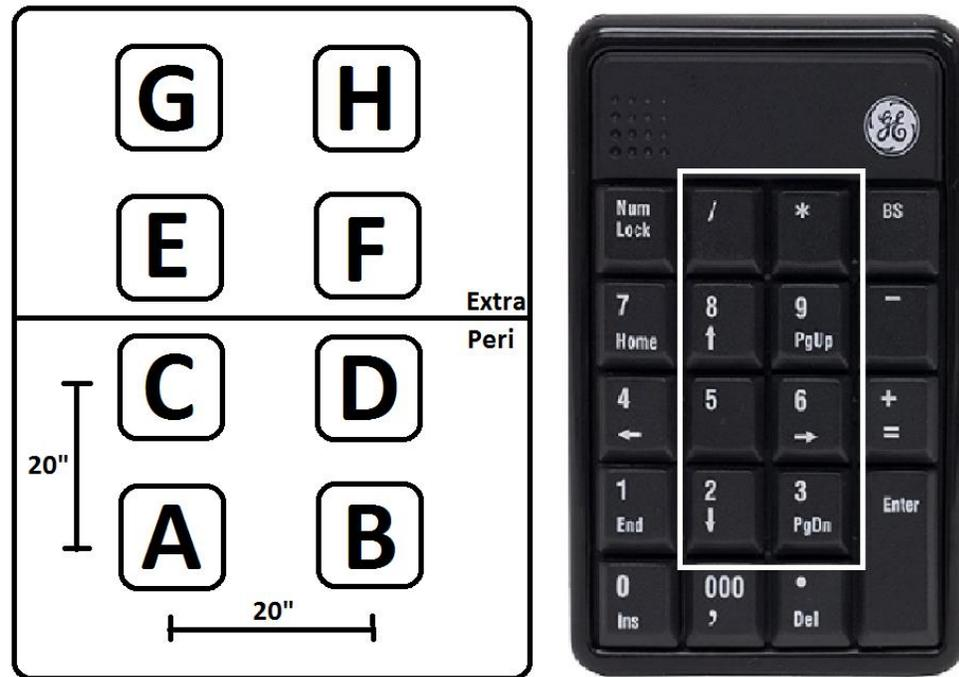
Figure 4- Schematic of speaker and response mechanism layout
