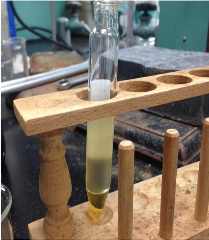
**Figure 2:** Wheat germ oil shows two layers the top layer is wheat germ methyl ester (Biodiesel) and the bottom layer is glycerin.
