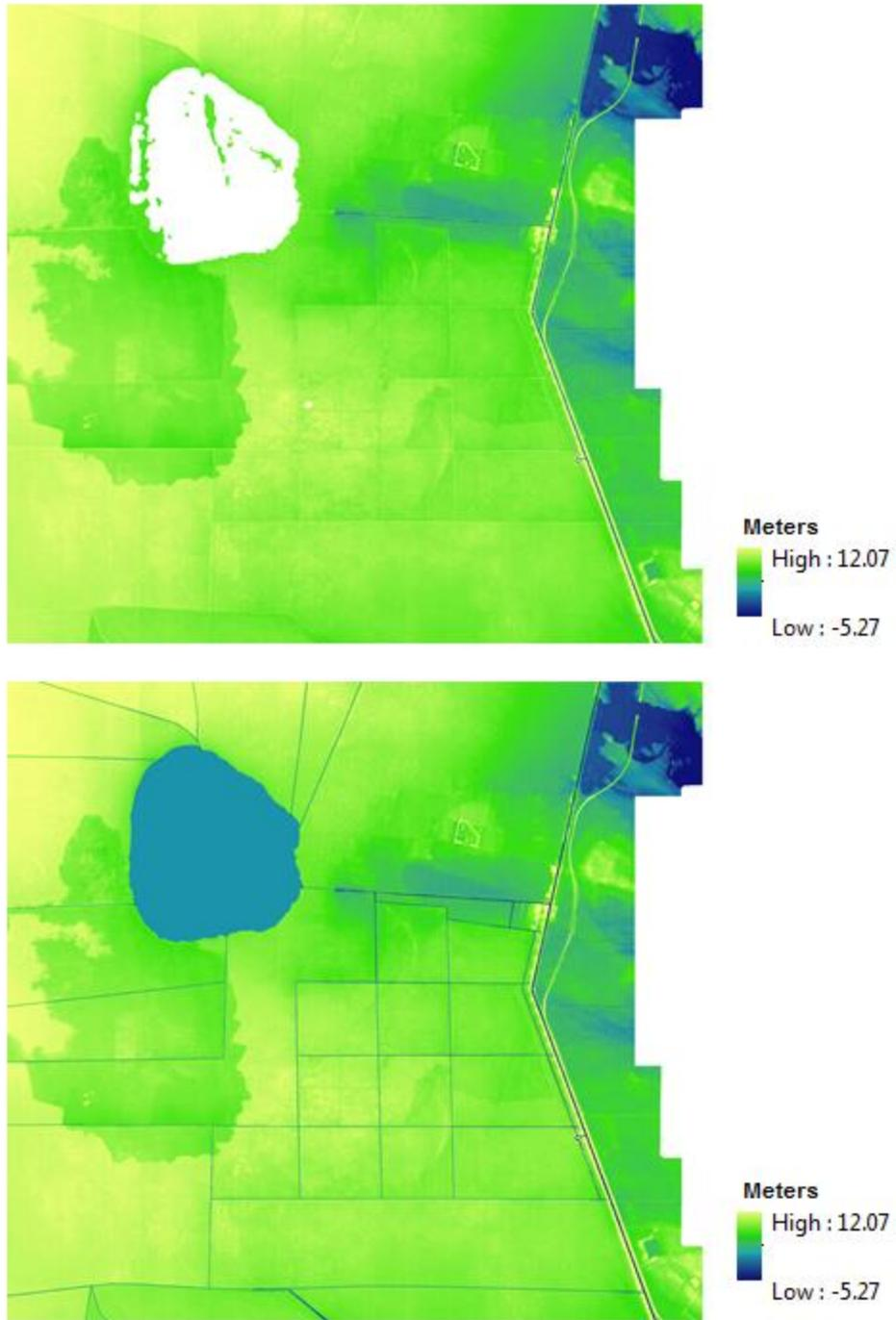
Figure 1 Subset of raw DEM without hydrologic conditioning (top) and hydroDEM after conditioning (bottom)
