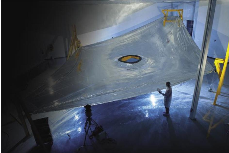
Figure 4.1: NeXolve Corporation is using NASA-derived thin films to construct the five-layer sunshields—one of which is shown here on a test fixture—for the James Webb Space Telescope. Image courtesy of Northrop Grumman Aerospace Systems
