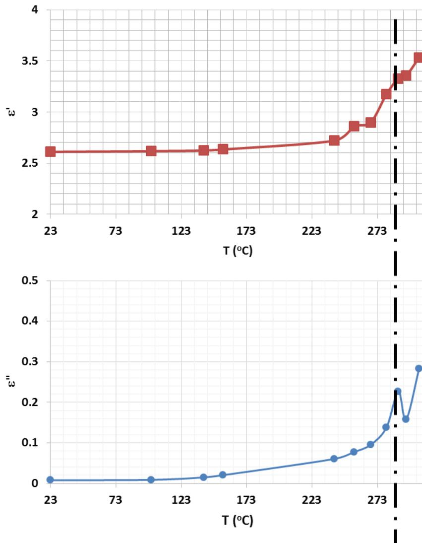
Figure 4.11: Real ( $\epsilon'$ ) and Imaginary ( $\epsilon''$ ) part of dielectric permittivity versus temperature.
