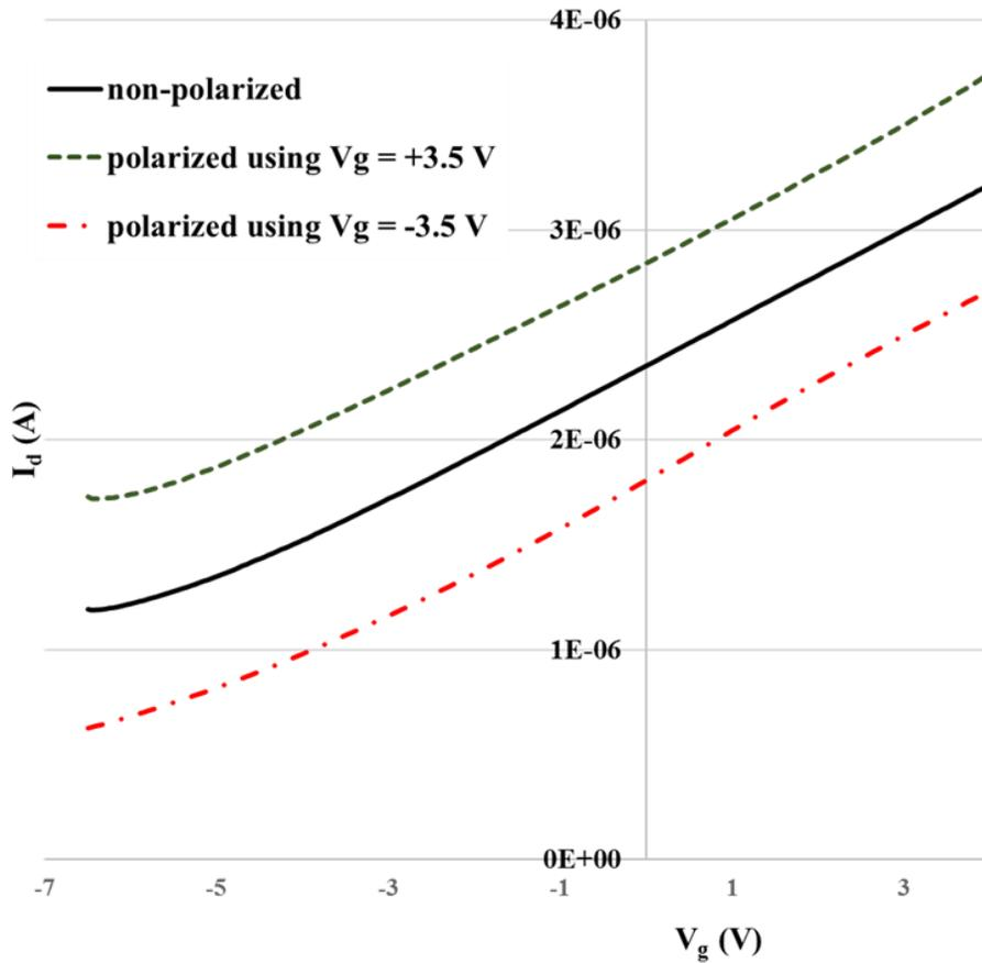
Figure 8.4:  $I_d - V_g$  characteristics of a  $2.5 \times 2.5 \mu\text{m}^2$  device in the unpolarized state (solid line), positively polarized using a positive bias of 3.5 V (dashed line), and negatively polarized using a negative bias of 3.5 V (dashed dot line).
