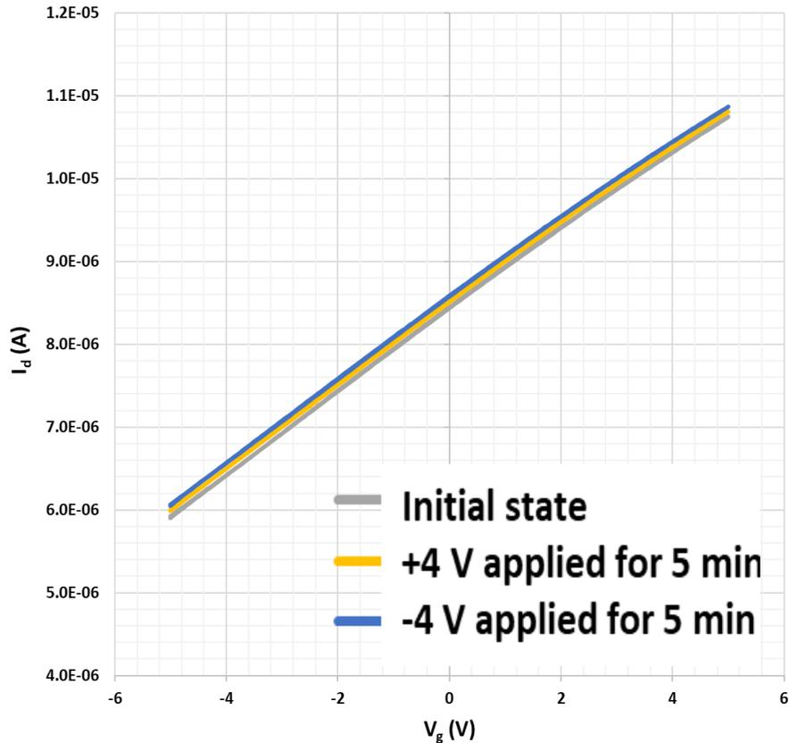
Figure 8.3: Attempt to program the device at room temperature
