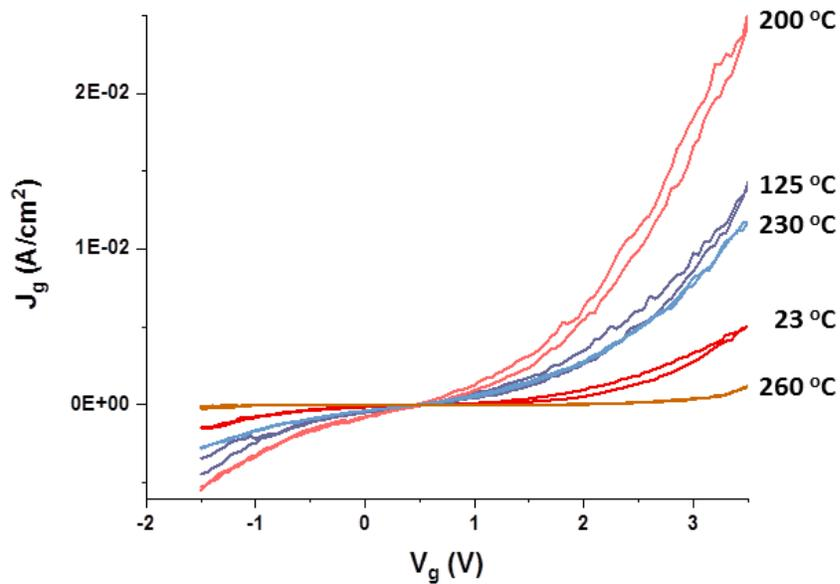
Figure 6.1: Heating of a virgin device with channel  $L = 3 \mu\text{m}$ ,  $W = 3 \mu\text{m}$ : leakage current density versus gate voltage in a linear scale.
