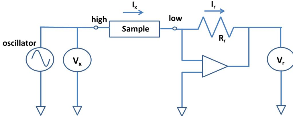
Figure 2.5: Principle of auto-balance bridge.
