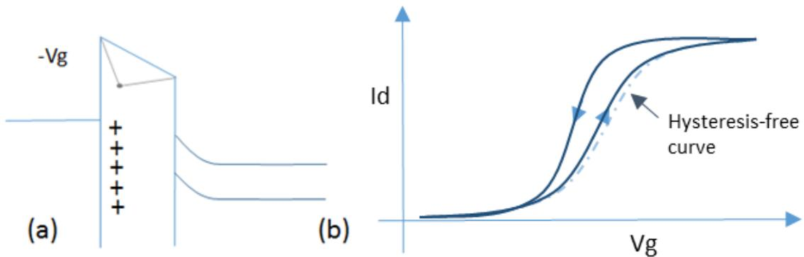
Figure 7.6: band bending and  $I_d$ - $V_g$  hysteresis caused by the presence of positive mobile ions.
