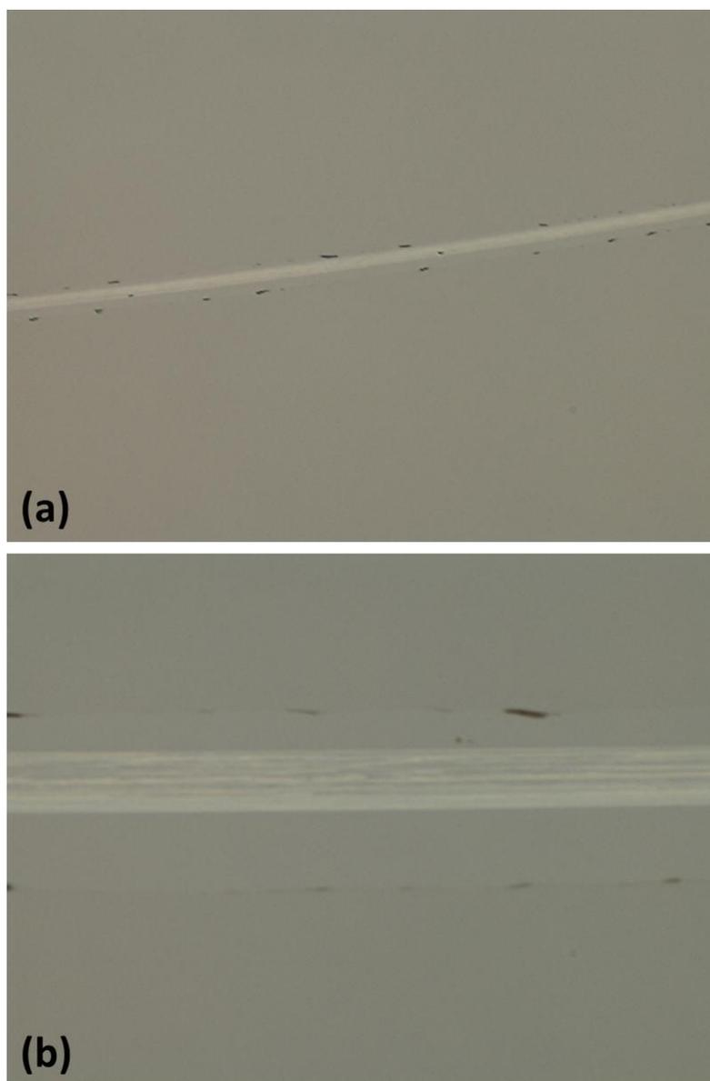
**Figure 4.5: Spin-coated continuous LaRC-CP1 film on Si (a) x20 , (b) x100 magification.**
