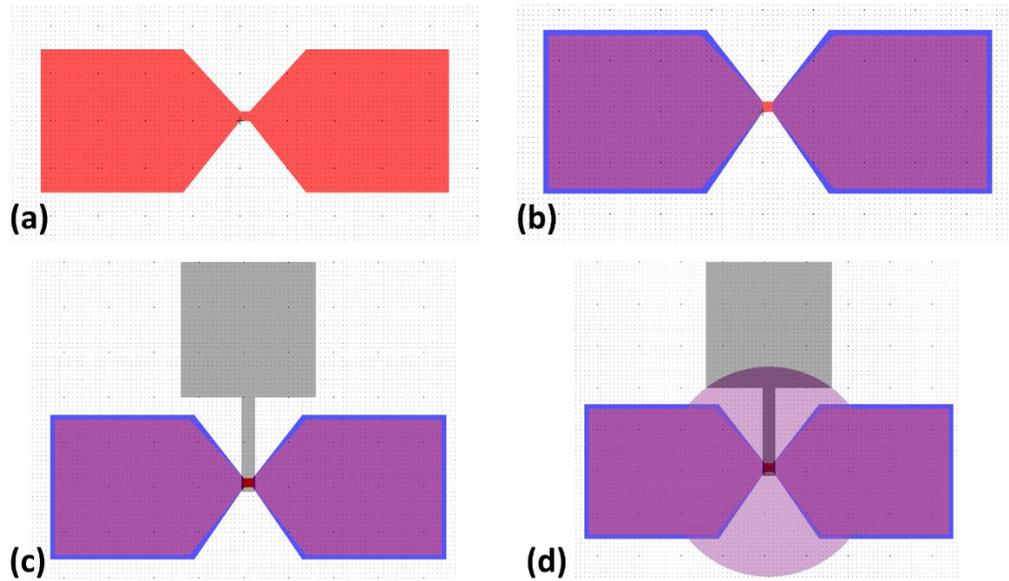
**Figure 5.2: Masks used for FeFETs fabrication (a) formation of channel and source and drain, (b) mask for lift-off process for the source and drain metal pads, (c) etching mask for gate electrode, and (d) shadow mask for device encapsulation.**
