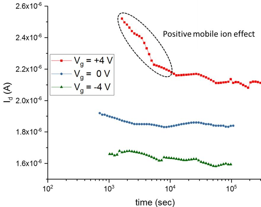
Figure 8.8: Memory retention measurements versus time.
