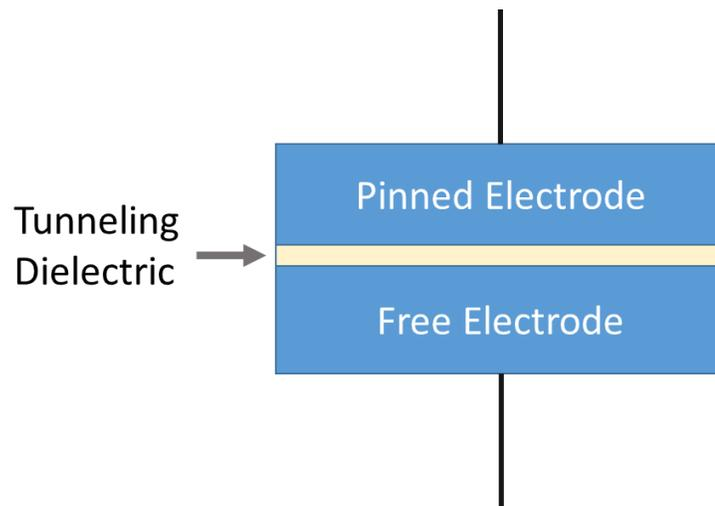
**Figure 1.5: Schematic of the MTJ in a STT-MRAM.**
