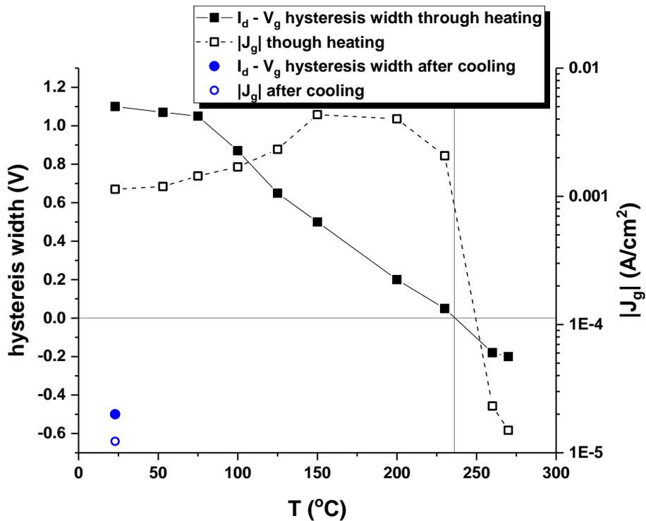
Figure 6.3: Evolution of leakage current density (absolute value of current density at  $V_g = -1.2$  V for each temperature) and  $I_d - V_g$  hysteresis width through temperature. CW hysteresis loop is represented with a positive value, while the CCW one with a negative value, horizontal line indicates where hysteresis changes direction and vertical line indicates the temperature at which it happens.
