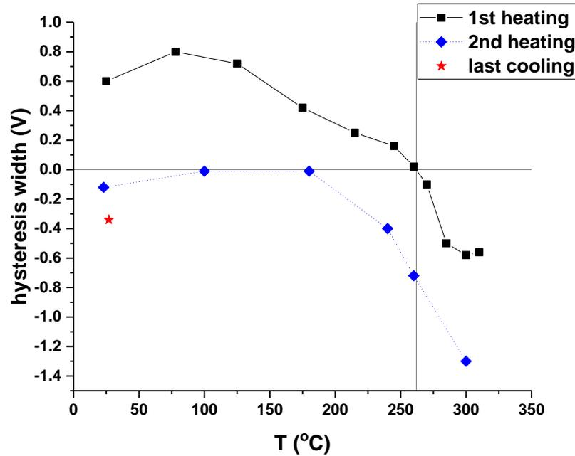
Figure 6.6: Hysteresis width vs. temperature (horizontal line indicates where hysteresis changes direction and vertical line indicates the temperature at which it happens).
