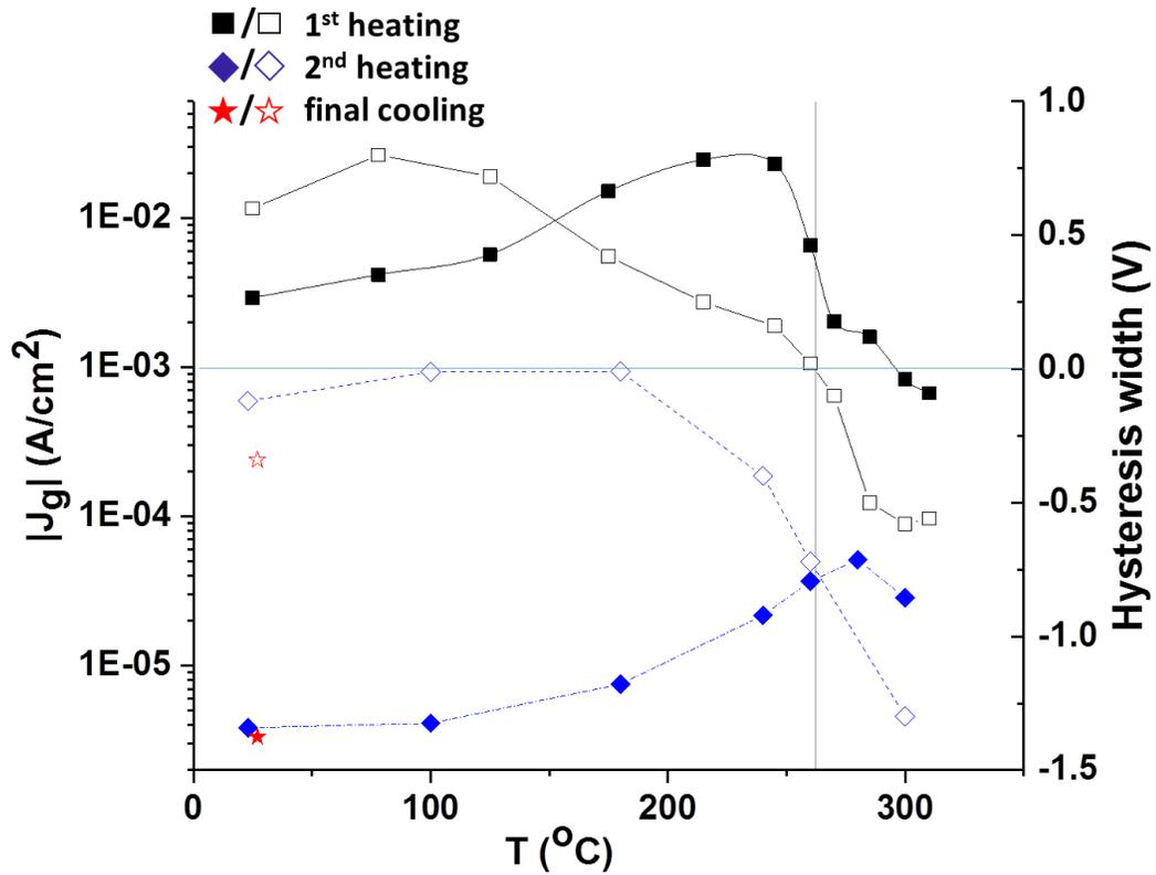
Figure 7.11: Leakage current density (filled symbols - absolute value of current density at  $V_g = -1.2$  V for each temperature) and hysteresis width (open symbols – largest hysteresis width of  $I_d$ - $V_g$  loop) development through temperature. Clockwise hysteresis loop is represented with a positive value, while the counter-clockwise one with a negative value, the vertical line indicates the temperature at which the hysteresis loop changes direction during the first heating cycle.
