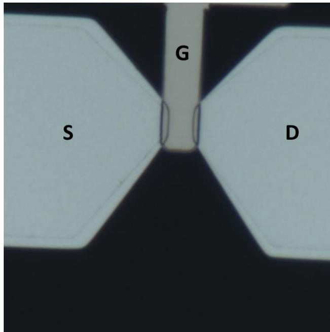
**Figure 5.4:** Optical microscope image of the fabricated device showing the gate-drain and gate-source overlap
