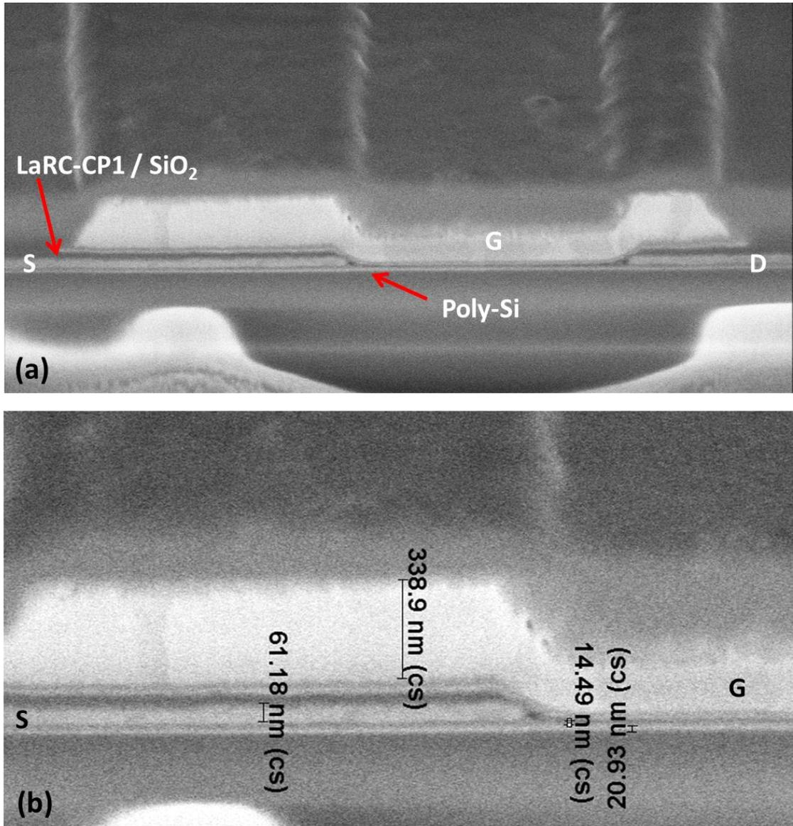
Figure 5.6. Cross-section of a fabricated device
