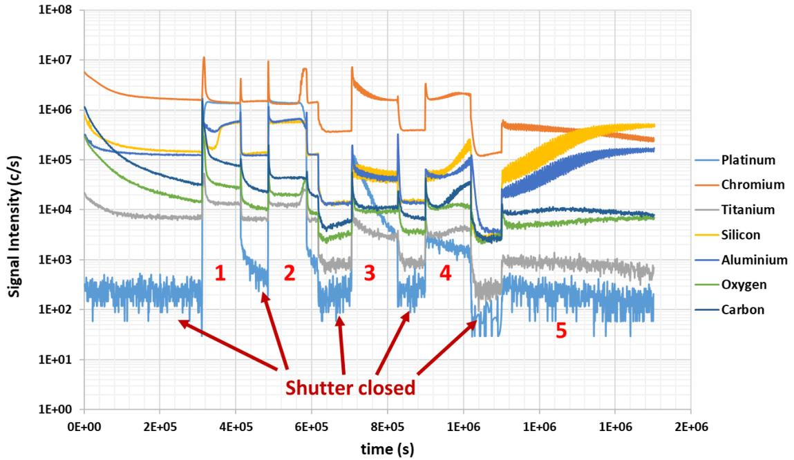
Figure 5.3: SIMS end-point detection
