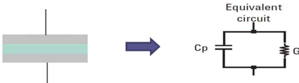
Figure 2.2: Dielectric capacitor and equivalent circuit.
