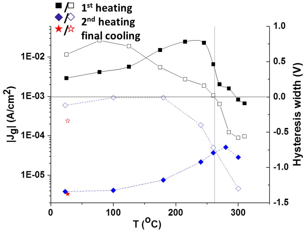
Figure 8.6: leakage current density (filled symbols - absolute value of current density at  $V_g = -1.2$  V for each temperature) and hysteresis width (open symbols – largest hysteresis width of  $I_d - V_g$  loop) evolution with temperature. Clockwise hysteresis loops are represented with positive values, while counter-clockwise loops are represented with negative values, the vertical line indicates the temperature at which the hysteresis loop changes direction during the first heating cycle.
