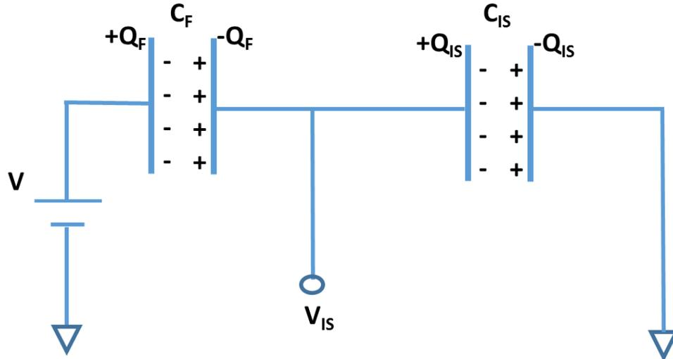
Figure 2.8: Gate stack represented of the FeFET transistor as a ferroelectric capacitance ( $C_F$ ) in series with the semiconductor capacitance ( $C_{IS}$ ).
