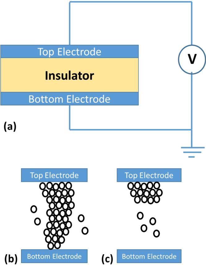
Figure 1.4: (a) RRAM cell schematic, (b) LRS, and (c) HRS.
