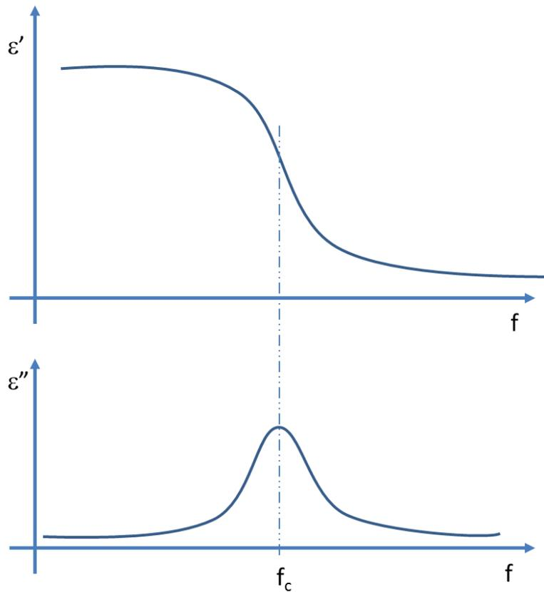
Figure 2.4: Dielectric Spectroscopy Measurements, frequency spectrum
