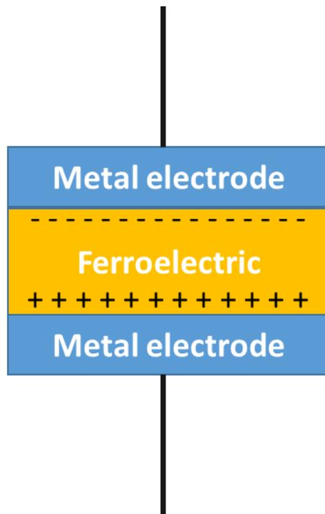
Figure 2.6: Ferroelectric capacitor memory cell.
