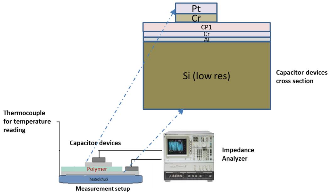
Figure 4.8: Samples and setup used for dielectric spectroscopy measurements.
