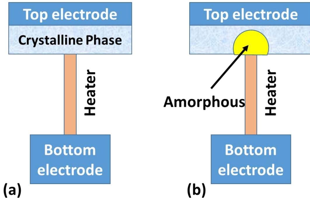
Figure 1.6: Cross-section of two PRAM memory cells: a) cell is in low resistance crystalline state, b) cell in high resistance amorphous state.
