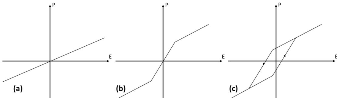
Figure 2.1: Polarization (P) versus applied electric field (E) in a (a) dielectric, (b) paraelectric, and (c) ferroelectric material
