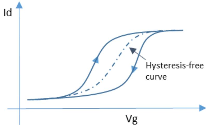
Figure 7.3:  $I_d$ - $V_g$  hysteresis loop resulting by charge-trapping injected from the semiconductor side.
