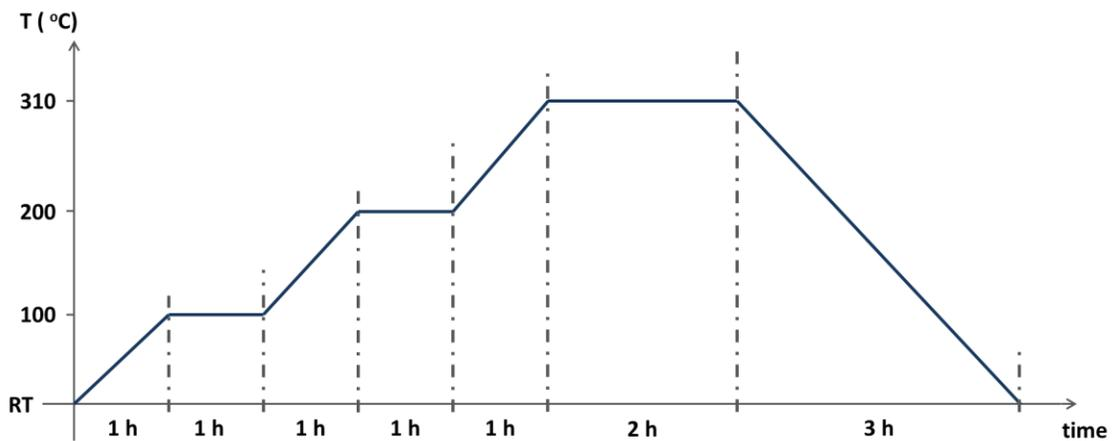
Figure 4.6: LaRC-CP1 curing process steps.
