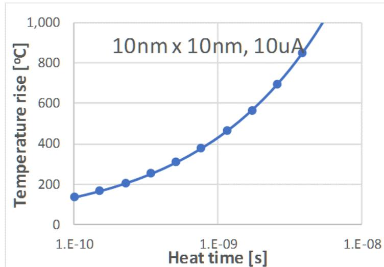
Figure 8.9: Simulated temperature rise of a 10 nm x 10nm transistor channel when 10  $\mu$ A current flows through.
