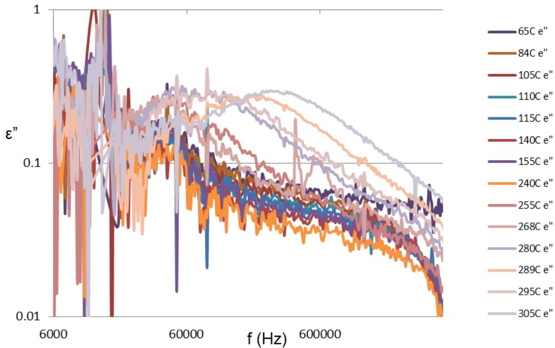
Figure 4.10: Measurement results of the imaginary part of dielectric permittivity.
