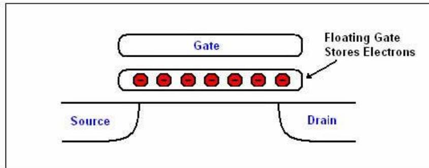
Figure 1.3: Flash memory floating cell
