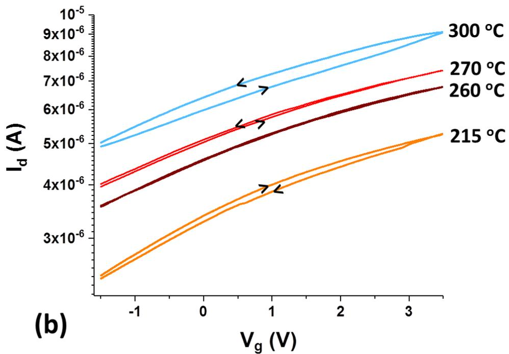
Figure 8.5: (a)  $I_d - V_g$  characteristics during the first heating cycle, (b) close-up of the high temperature range.
