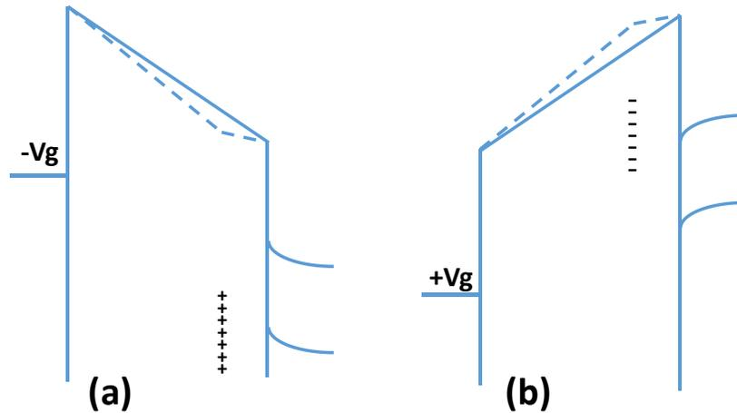
Figure 7.2: Effect of charge trapping on device band bending.
