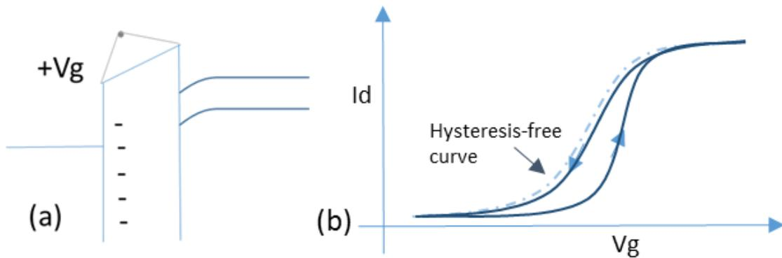
Figure 7.5: band bending and  $I_d$ - $V_g$  hysteresis caused by the presence of negative mobile ions
