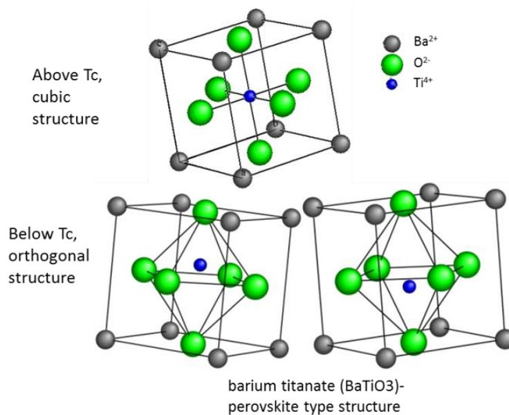
**Figure 2.9:  $BaTiO_3$  crystal structure, and the ion displacement.**
