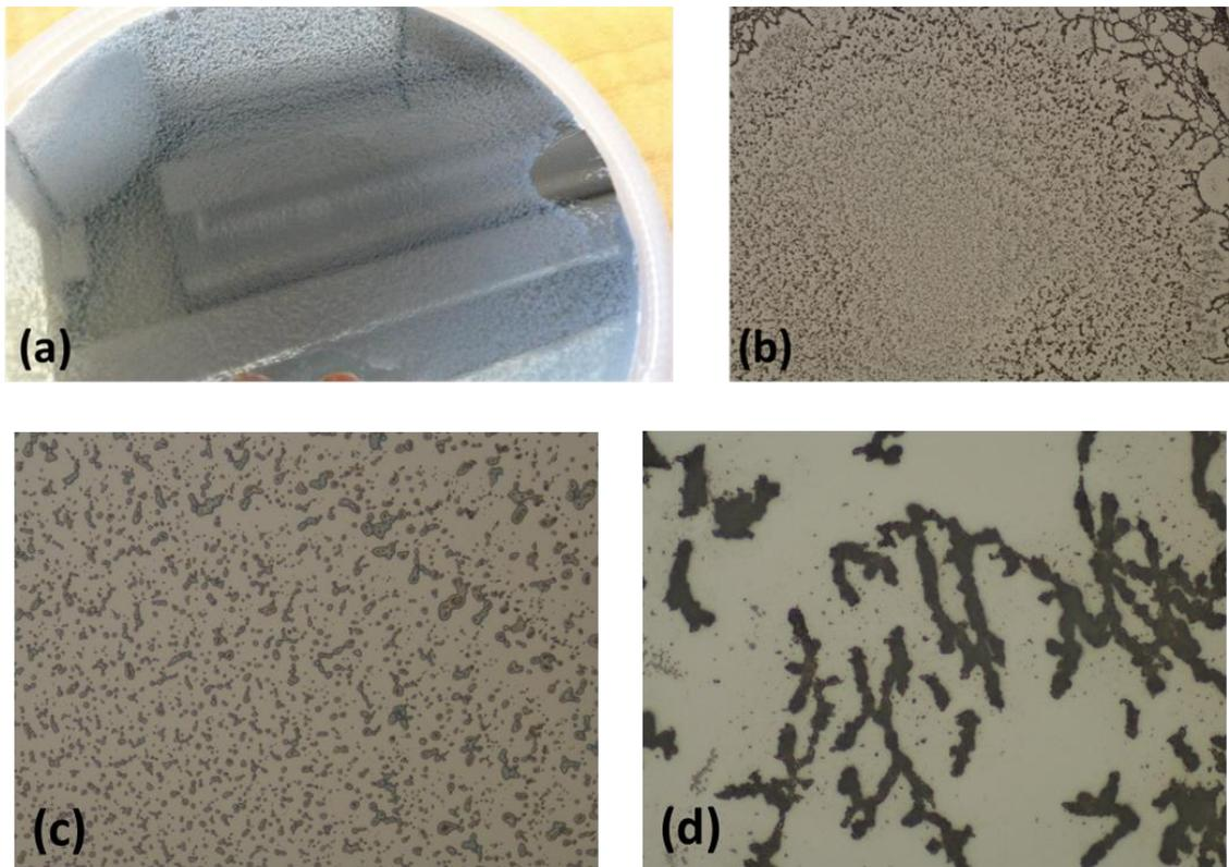
**Figure 4.3: Polymer agglomeration after spin-coating of a 3% LaRC-CP1 solution on Si at 2500rpm (a) photo of the wafer, and optical image through microscope (b) x5, (c) x20, and (d) x50 magnification .**
