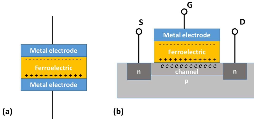
Figure 1.7: (a) Ferroelectric Capacitor, and (b) Ferroelectric Transistor.
