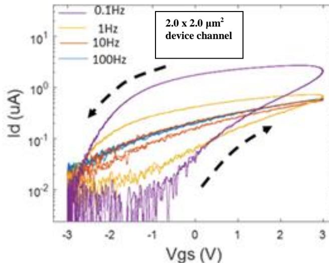
Figure 7.8:  $I_d$ - $V_g$  hysteresis at corresponding frequencies
