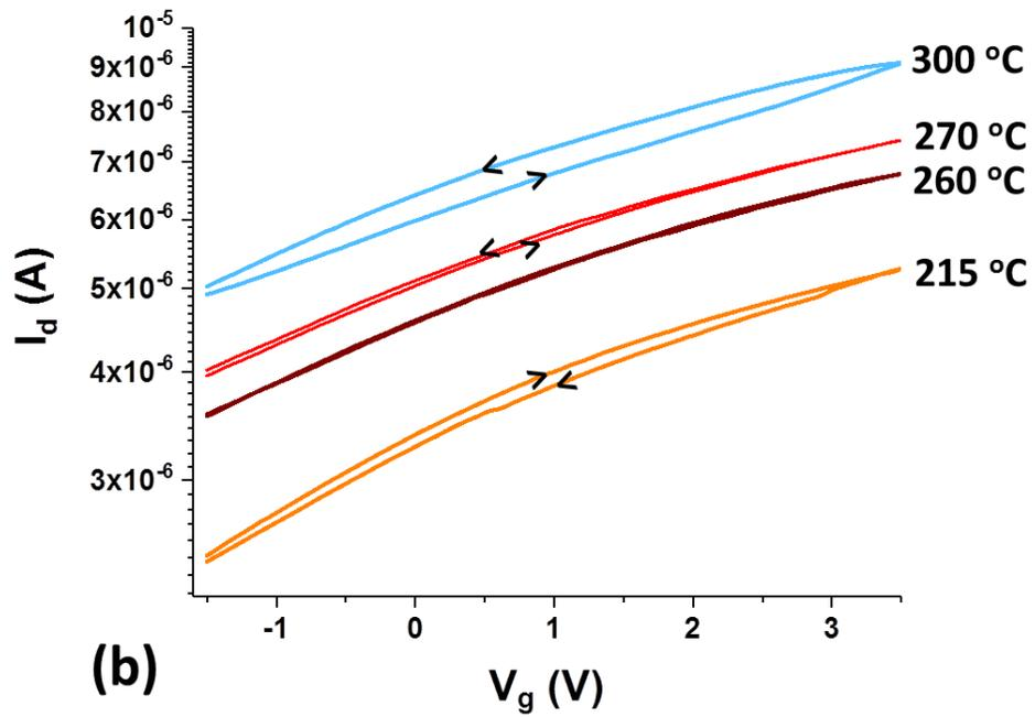
Figure 7.10:  $I_d - V_g$  characteristics during a heating cycle
