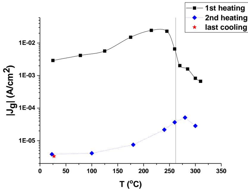
Figure 6.5: Leakage current density vs. temperature in semi-log scale (vertical line indicates temperature at which hysteresis loop changes direction). Device channel  $L = 3 \mu\text{m}$ ,  $W = 3 \mu\text{m}$ .
