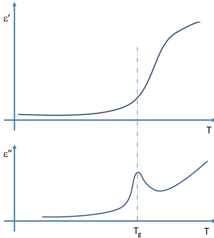
**Figure 2.11: Dielectric Spectroscopy Measurements, temperature spectrum**
