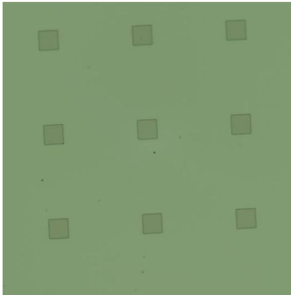
Figure 4.7: Microscope image of an array of fabricated capacitors.
