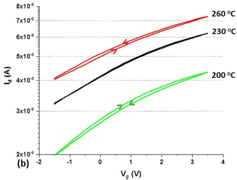
Figure 6.2: Heating of a virgin device with channel  $L = 3 \mu\text{m}$ ,  $W = 3 \mu\text{m}$ : (a)  $I_d$ - $V_g$  characteristics in a semi-log scale (direction noted by arrows), and (b) is an expanded scale view of the  $I_d$ - $V_g$  characteristics at the highest temperatures.
