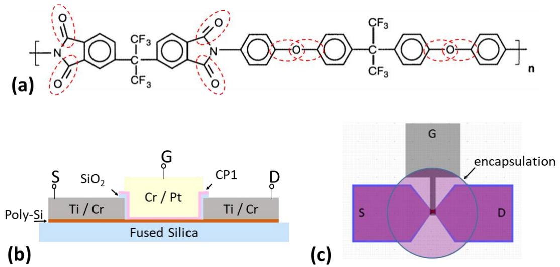
Figure 7.7: (a) LaRC-CP1 chemical structure, and fabricated devices cross-section (b) and layout (c).
