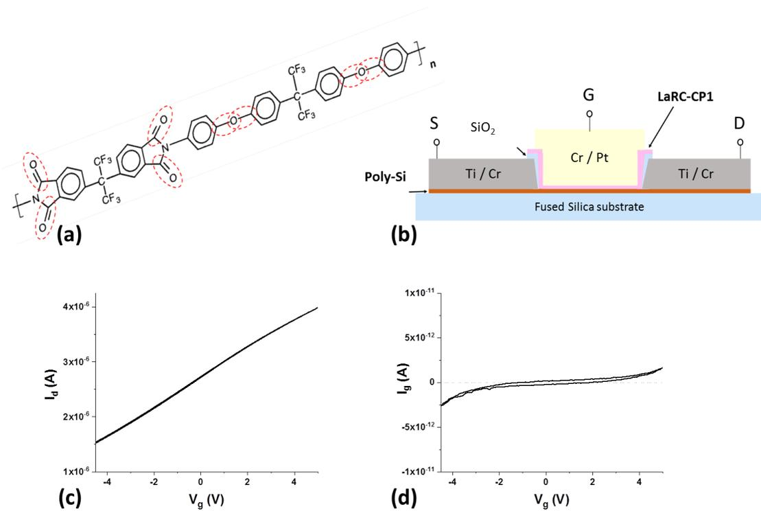
**Figure 8.1:** a) Chemical Structure of CP1 Polyimide molecule. Dashed ovals designate the dipoles believed to contribute to the ferroelectric effect. b) Schematic cross-section of the device structure. c)  $I_d$ - $V_g$ , and d)  $I_g$ - $V_g$  characteristics for a device with channel  $L = 2.5 \mu\text{m}$  and  $W = 2.5 \mu\text{m}$ .
