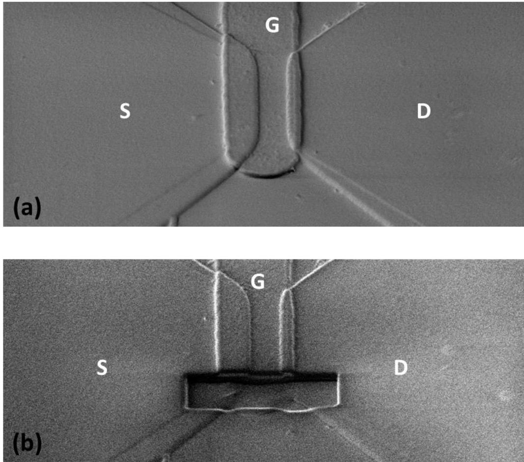
**Figure 5.5 (a) SEM image of device top view, (b) device top view after FIB**
