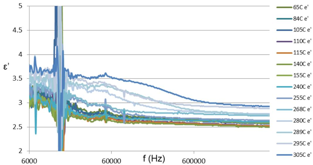
**Figure 4.9: Measurement results of the real part of dielectric permittivity.**
