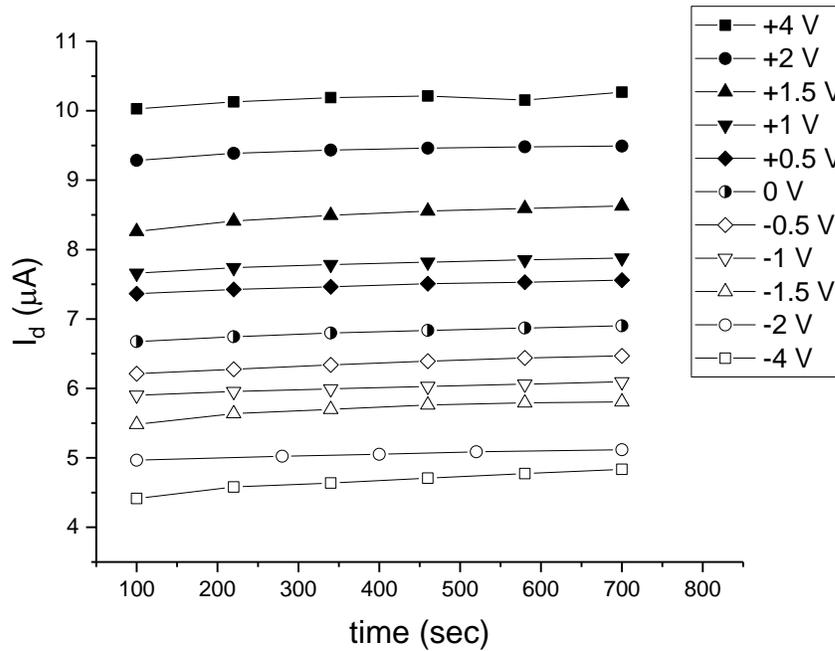
Figure 8.7: Multi-state memory effect for a device with channel  $L = 2 \mu\text{m}$ , and  $W = 6.5 \mu\text{m}$ .
