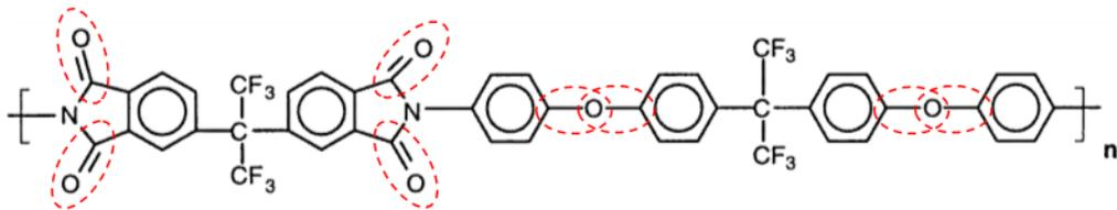
Figure 4.2: Chemical structure of LaRC-CP1 polyimide molecule.
