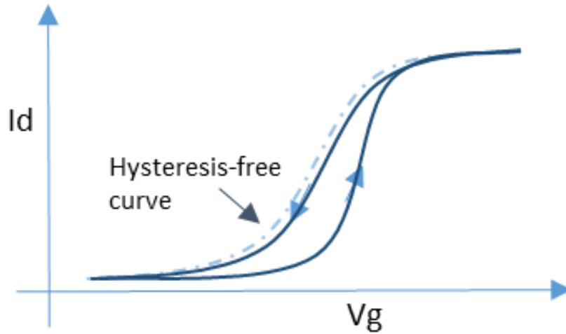
Figure 7.4:  $I_d - V_g$  hysteresis loop resulting by charge-trapping injected from the metal gate electrode side.
