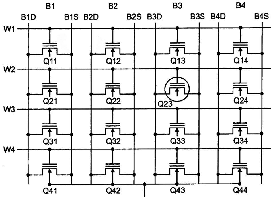
Figure 3.1: Example of memory cell array.
