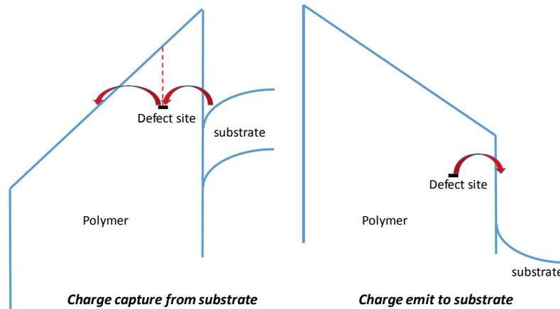
**Figure 6.4:** Schematic drawing of the device band diagram illustrating the charge capture process.
