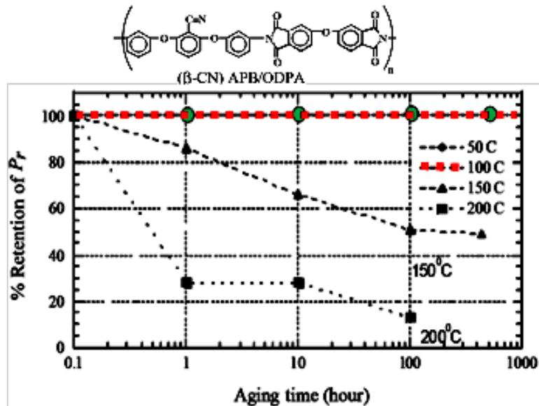
Figure 3.2: Example of polarization retention for a high  $T_g$  polymer.
