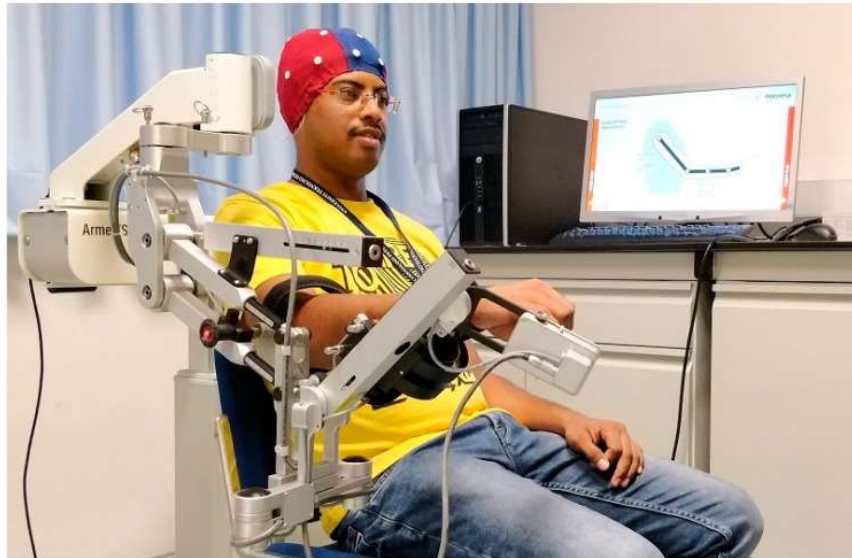
Figure 3: Upper limb (ArmeoSpring) at SMART Lab, UTP. 1 Multi-joint exoskeleton for shoulder, elbow and wrist joints with seven degrees of freedom controlled through a BMI based on MI-ERD of sensorimotor oscillations in the \beta -band.
