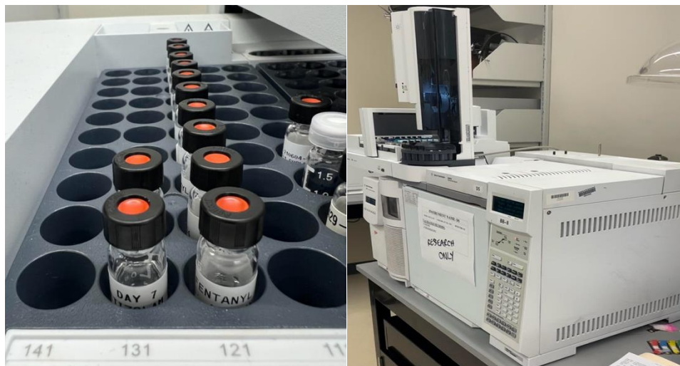
Figure 3. Autosampler vials were loaded on the GC-MS starting with the point calibrators following the syringe extracts (LEFT). GC-MS used for the research (RIGHT).
