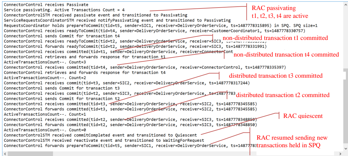
Figure 10.22 Fragment of the execution trace of reusable RAC during planned adaptation scenario
