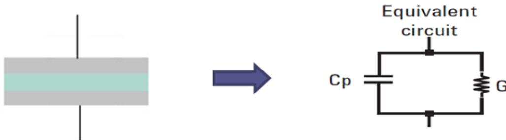
Figure 2.2: Dielectric capacitor and equivalent circuit.
