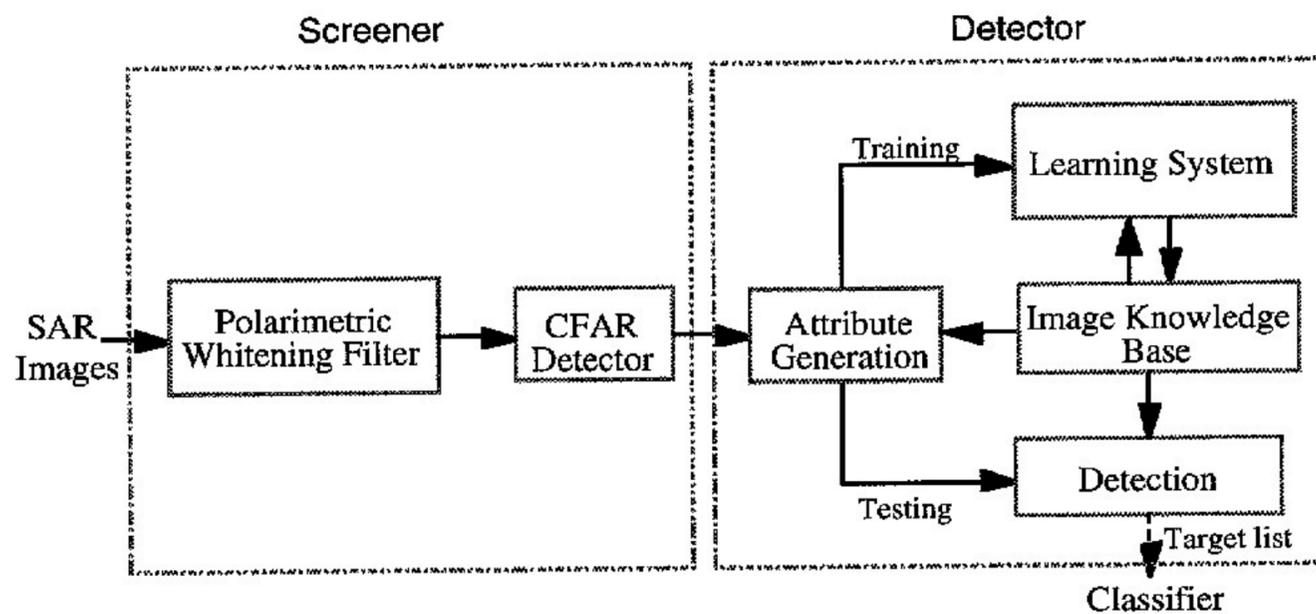
Figure 2. The system architecture.
