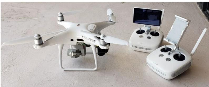
Figure 11. Phantom UAS and RCs.
