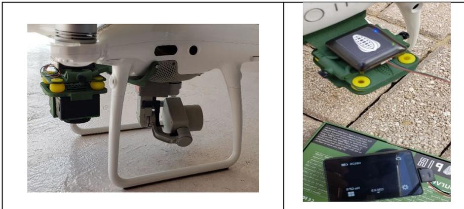
Figure 13. Phantom with MAPIR camera and GPS unit on mounting frame; Right: closeup of MAPIR GPS unit.
