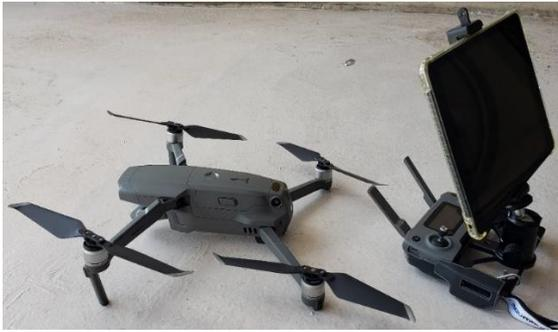
Figure 8. Mavic Pro 2, RC, and tablet (flight screen) used for this research.
