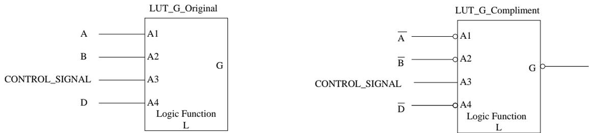
Figure 4.4: Complementing Control Logic
