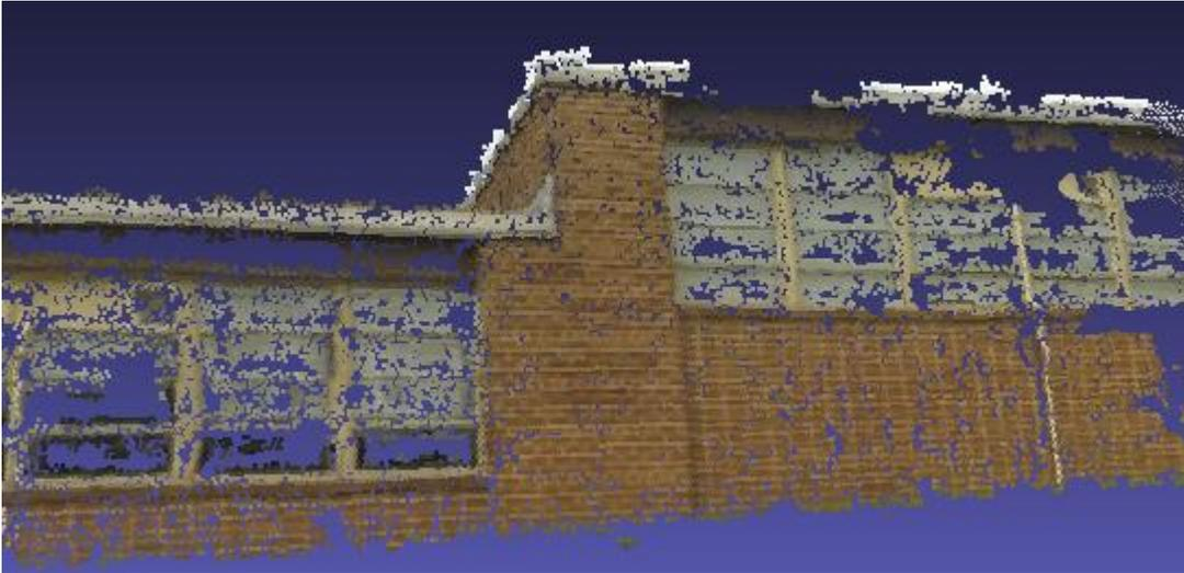
**Figure 18 - MeshLab: Dense point cloud**
