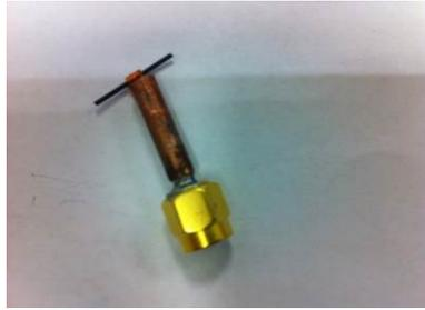
Figure 4.5: Handmade Coil Probe
