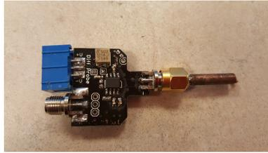
Figure 4.14: The Coil Probe with Differential Amplifier
