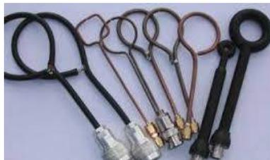
Figure 4.3: Coaxial Cable Probe
