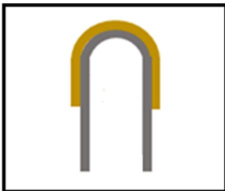
Figure 3.6 Convex bending of PET/Au. (■ PET Membrane, ■ Gold).
