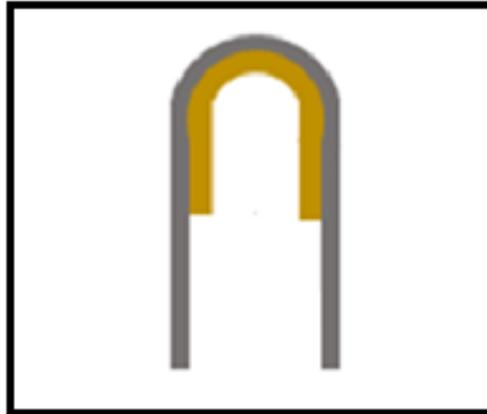
Figure 3.10 Concave bending of PET/Au. (■ PET Membrane, ■ Gold).
