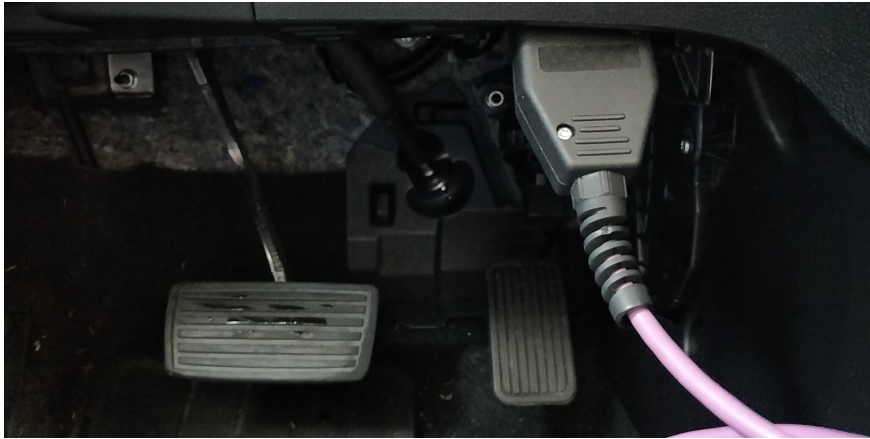
Figure 4.6: ODB-II port location on experiment vehicle
