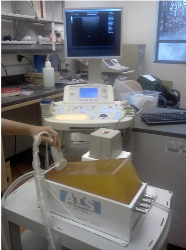
**Figure 15: Doppler Phantom scanning for reconstruction**
