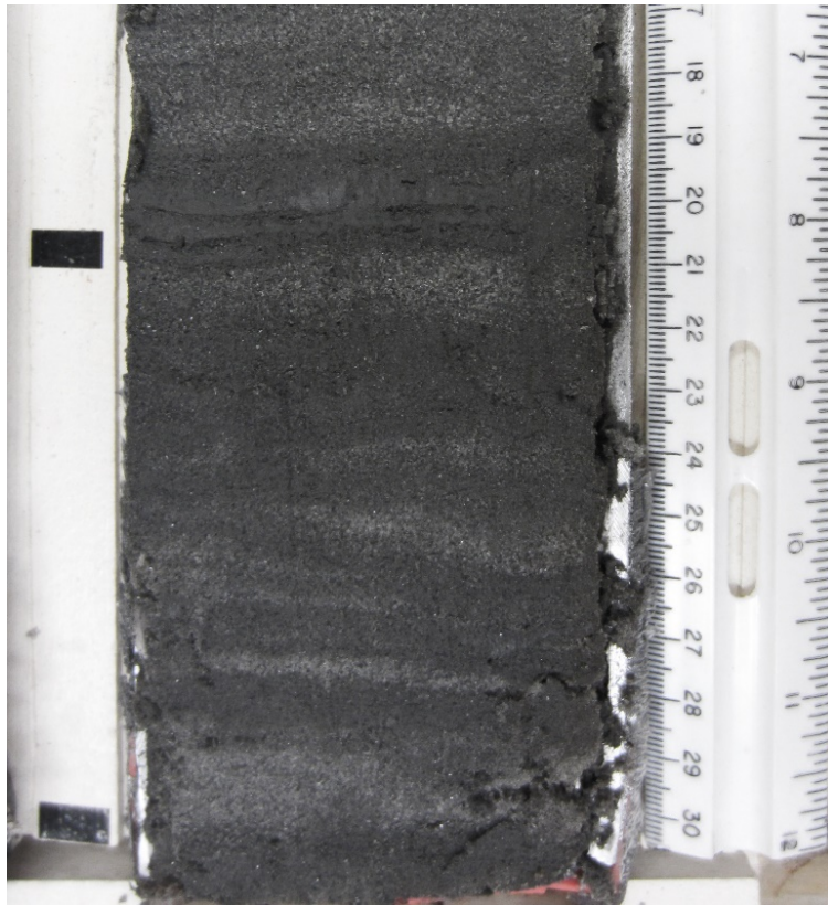
Figure 107: Close up of lenticular bedding. This image is from the 287 to 300 cm interval of core SI-14-02.
