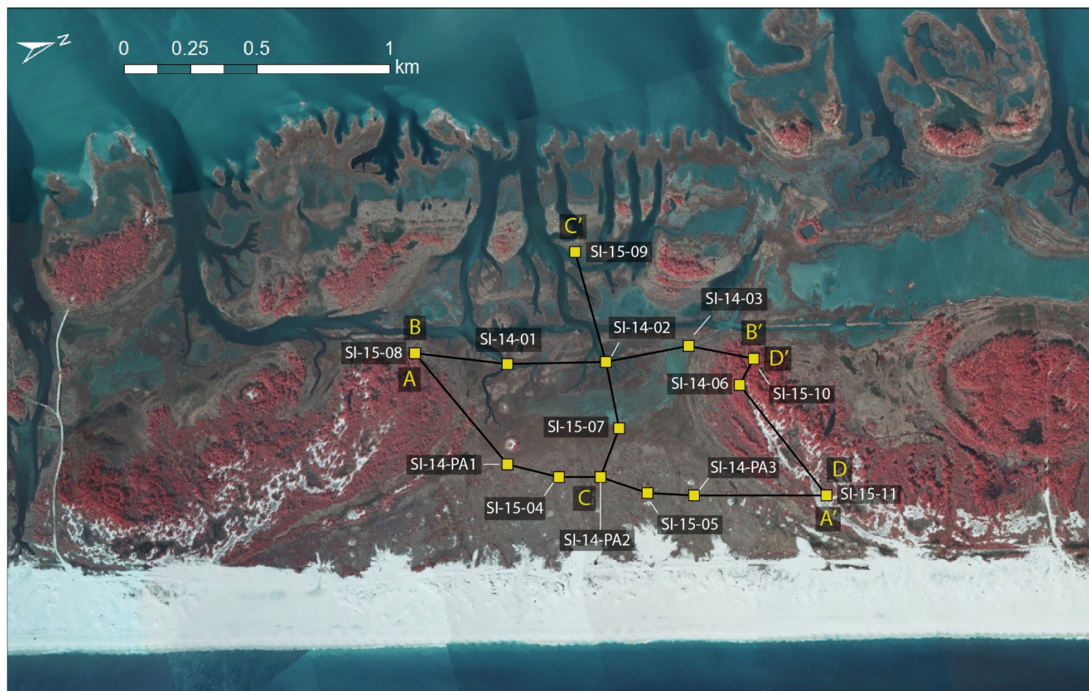
Figure 72: The former Sinepuxent Inlet showing sediment core locations and geologic cross section transects.
