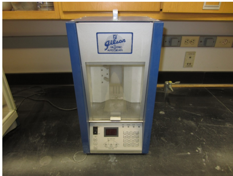
Figure 36: The Gilsonic Auto Siever used for sediment grain-size analysis.
