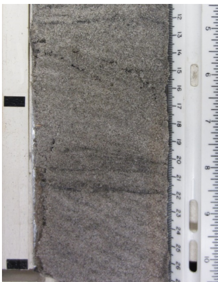
Figure 89: Close up of cross-laminated features truncated by planar-laminated features within core GR-15-09 from the 185 to 200 cm interval.
