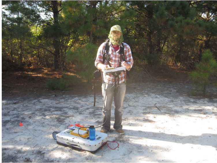
Figure 30: An image of the Mala 250 MHz GPR antenna employed for this study.
