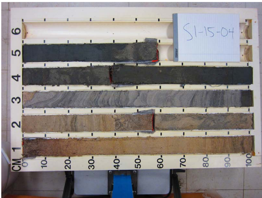
Figure 35: Example of a vibracore cut into 1-meter sections, split open longitudinally, and photographed.
