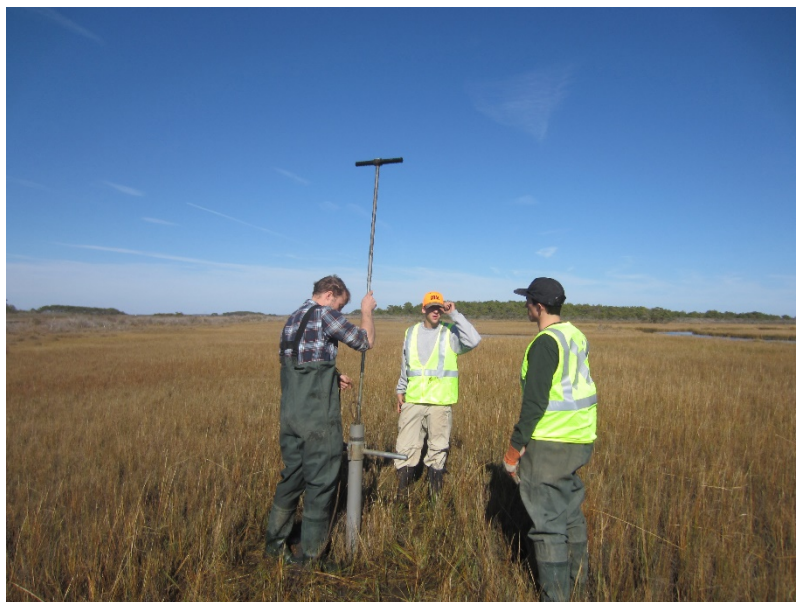
Figure 34: An image showing collection of a sediment core with the Eijkelkamp bailer borer system (pulse auger) technique.
