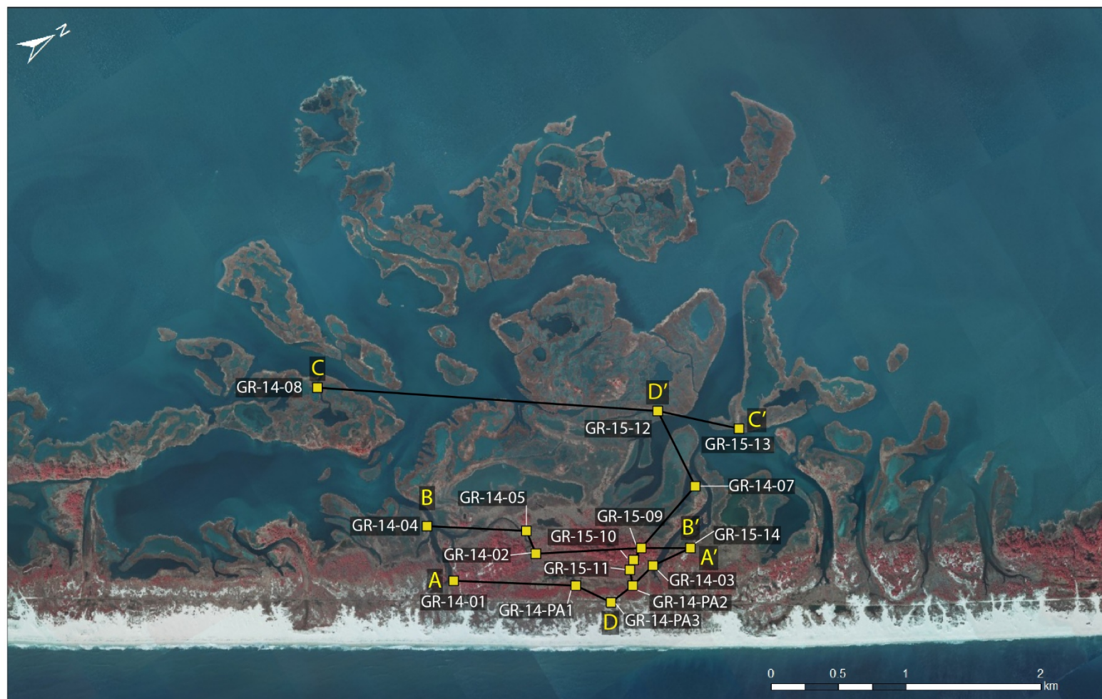
Figure 71: The former Green Run Inlet area showing sediment core locations and geologic cross section transects.
