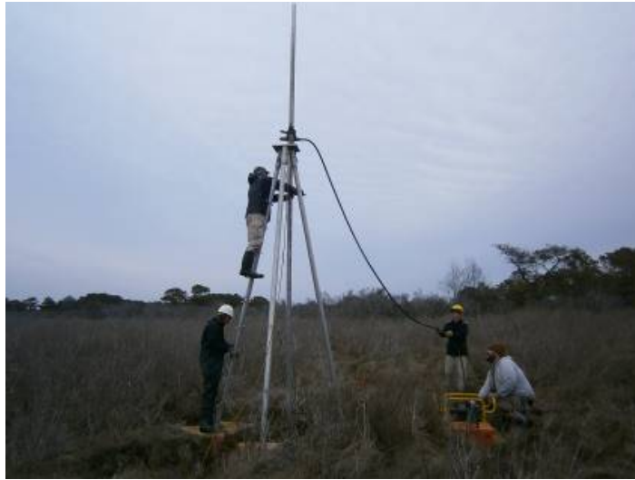
Figure 33: An image demonstrating the collection of a sediment core with the vibracore technique.
