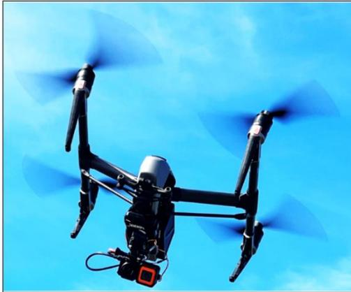
**Figure 1: The primary air-based platform used for this research (the DJI Inspire 2) carrying the RGB-LWIR payload.**
