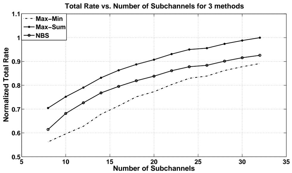
Figure 2.14: A comparison of the allocated rate per user for different number of subchannels the Max-Min, Max-Sum, and the proposed algorithm ( $K = 8$ )
