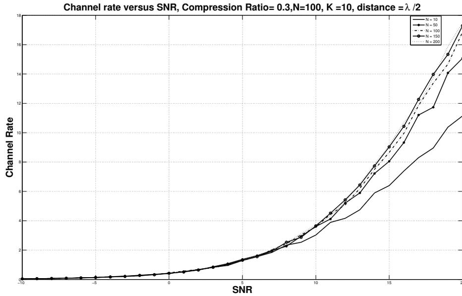
Figure B.7: Channel rate with compressed information for different numbers of BS antennas  $N$
