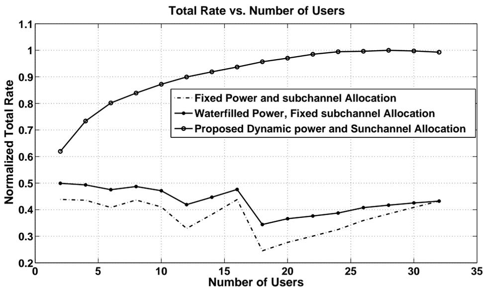
Figure 2.11: A comparison of fixed subchannel and power assignment, waterfilling power, and the proposed algorithm for  $N = 32$  subchannels
