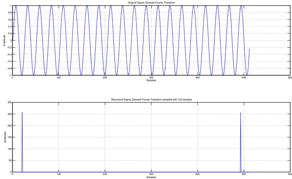
Figure B.2: Recovered sinusoid from compressed samples
