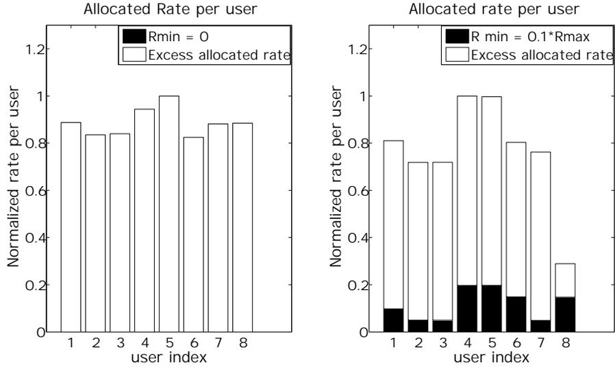
Figure 2.15: Allocation of minimum rate and the excess subchannels ( $N = 128$ ,  $K = 8$ )
