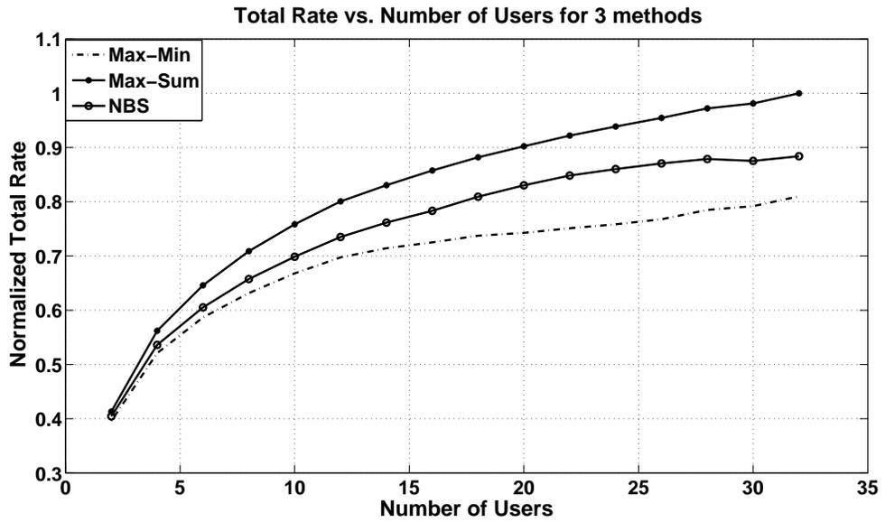
Figure 2.13: A comparison of the allocated rate per user for the Max-Min, Max-Sum, and the proposed algorithm ( $N = 32$ )
