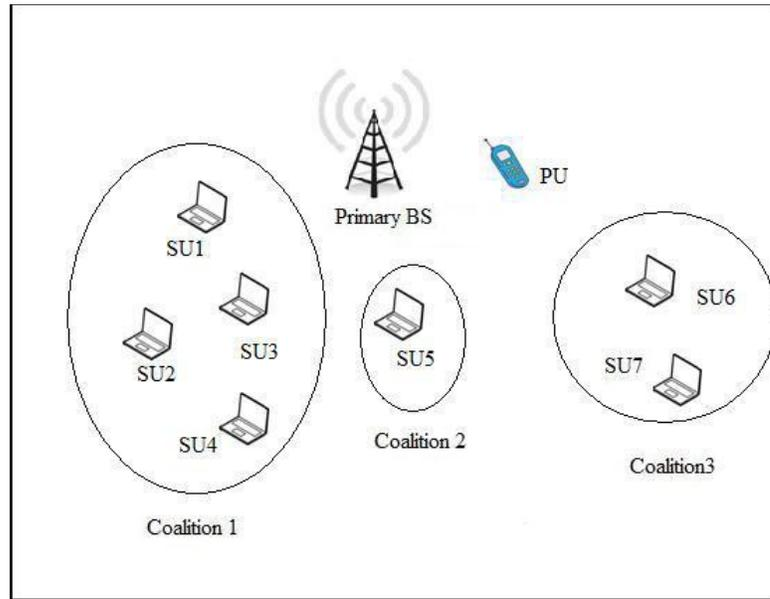
Figure 3.3: Distributed spectrum sensing
