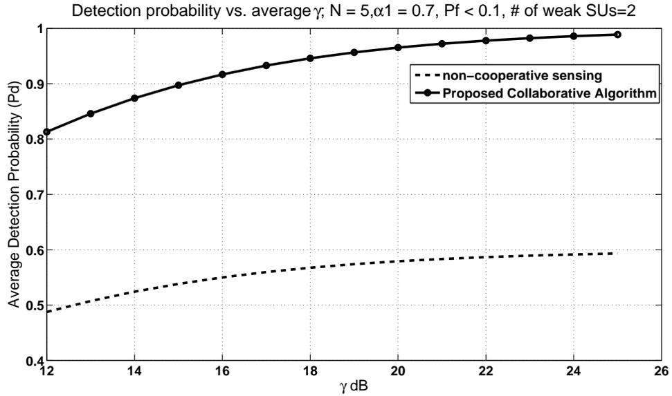
Figure 3.7: The average detection probability for the case of proposed collaborative algorithm (-o) and non-cooperative case(-).  $N = 5$ ,  $P_f = 0.1$ ,  $\alpha_1 = 0.7$ ,  $n_w = 2$
