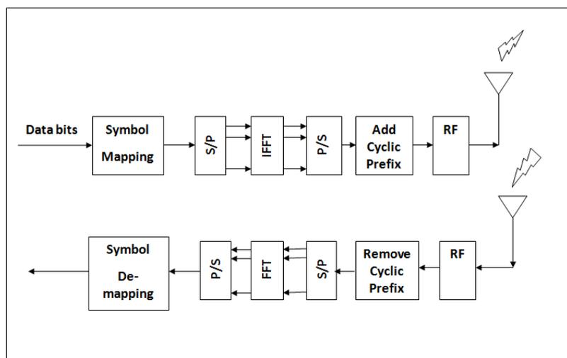
Figure 1.1: OFDM block diagram
