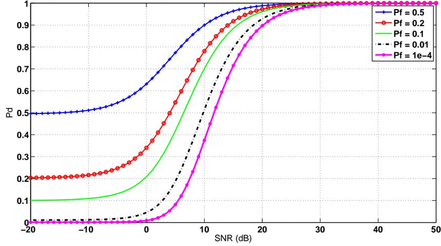
Figure 4.4:  $p_{d,i}$  vs  $SNR$  for different values of  $P_f$ ,  $p_p = 0.3$
