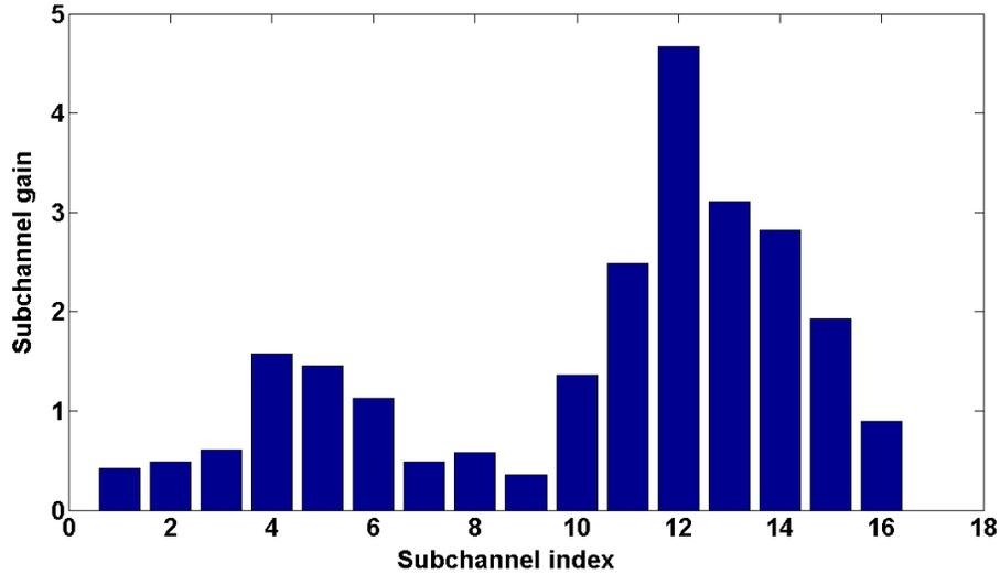
Figure 2.1: The effect of a frequency selective channel on subcarriers of an OFDM signal
