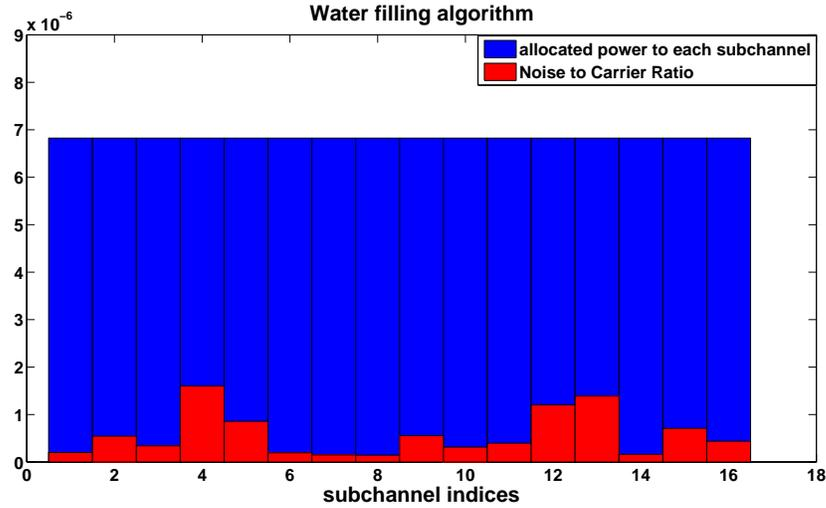
Figure 2.4: Power water filling for the case of single user,  $N = 16$  subchannels, and  $P_{max} = 0.1$  mW
