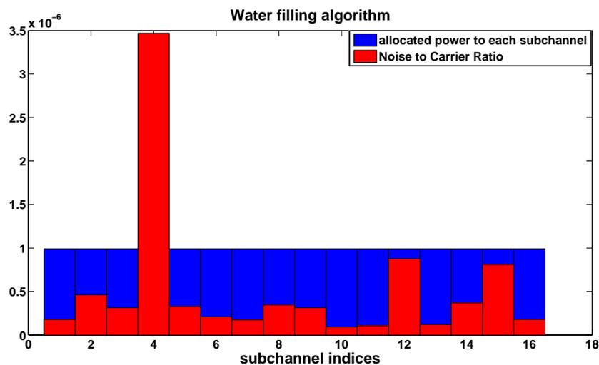
Figure 2.3: Power water filling for the case of single user,  $N = 16$  subchannels, and  $P_{max} = 0.01$  mW
