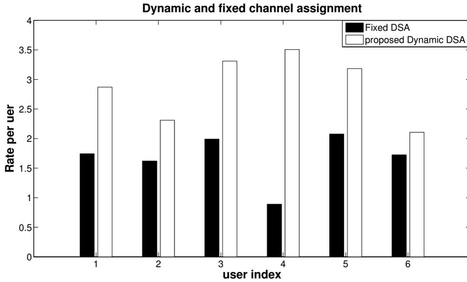
Figure 2.10: A comparison of fixed subchannel assignment and the proposed algorithm ( $N = 16$ ,  $K = 6$ )
