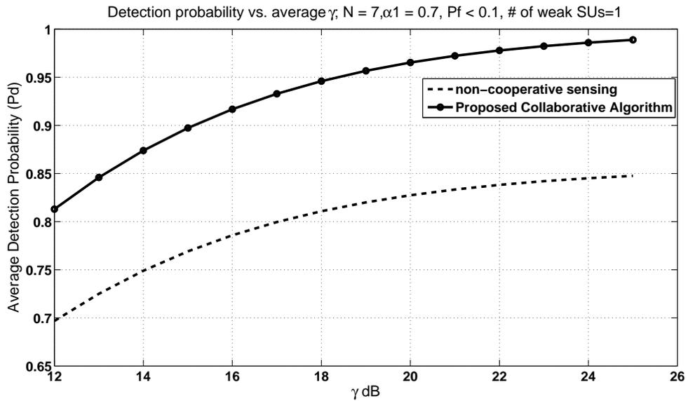
Figure 3.8: The average detection probability for the case of proposed collaborative algorithm (-o) and non-cooperative case(-).  $N = 7$ ,  $P_f = 0.1$ ,  $\alpha_1 = 0.7$ ,  $n_w = 1$
