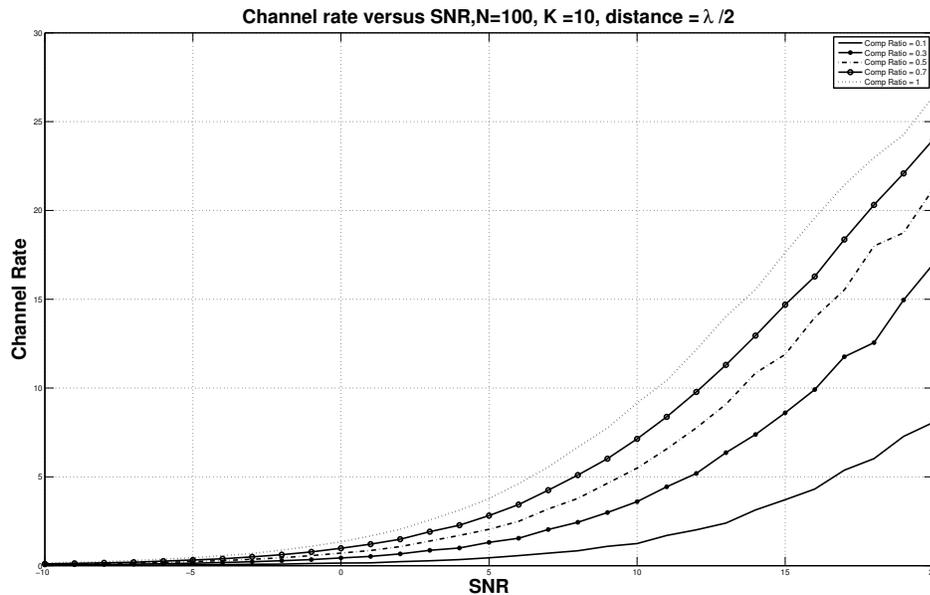
Figure B.6: Channel rate with perfect and compressed information for different compression ratios
