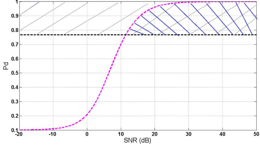
Figure 4.5:  $p_{d,i}$  vs  $SNR$ ,  $Pf = 0.1$ ,  $p_p = 0.3$ ,  $\beta_T \geq 0.9$
