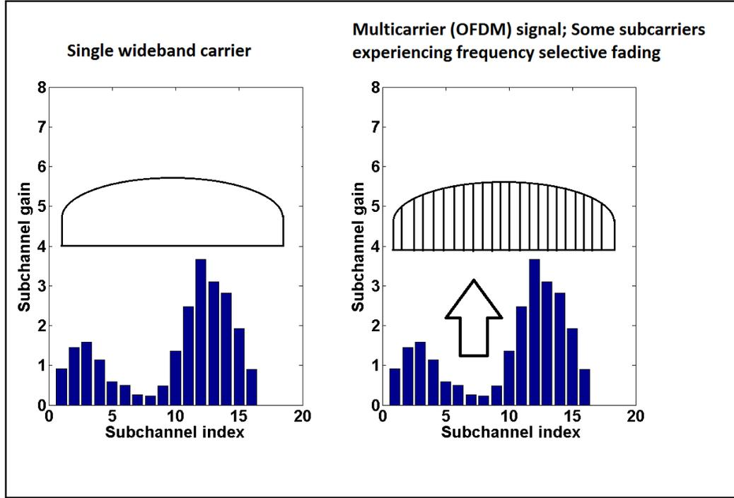
Figure 2.2: Transmission of a wideband single carrier signal vs multi-carrier (OFDM) over a frequency selective
