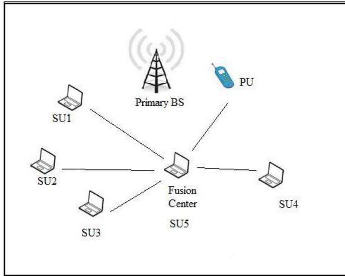
Figure 3.2: Centralized spectrum sensing
