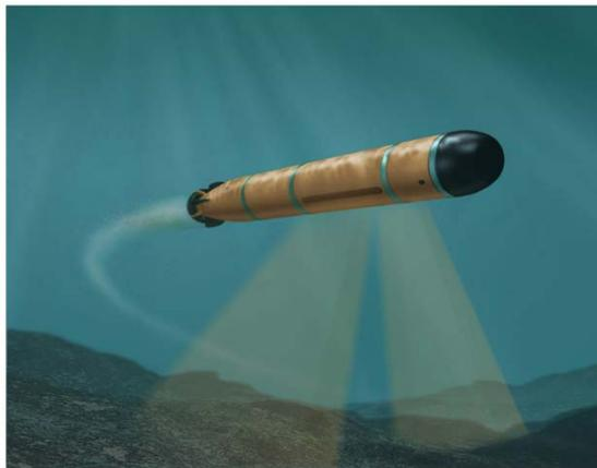
Figure 1.1 Typical Torpedo Shaped AUV (source: [www.asftauv.com](http://www.asftauv.com))
