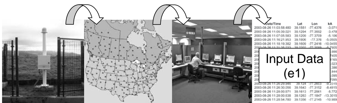
Figure 6.3 Vaisala’s Lightning Strike Input Data Flow Path ( www.vaisala.com )
