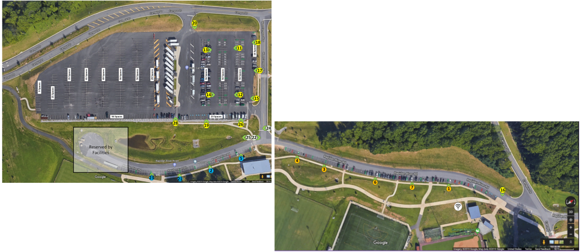
Figure 8.1: Lot Node Placement, Primary Campus WiFi Uplink
