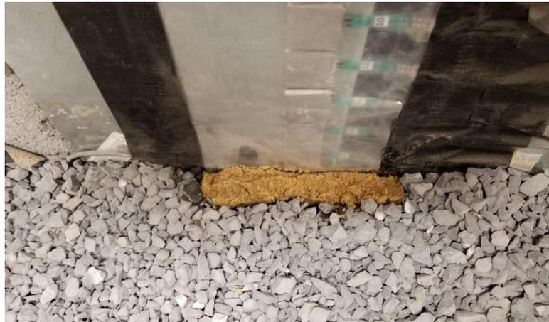
**Figure 4: 25mm thick sand interface in between AASHTO No. 8 aggregate and FSR**
