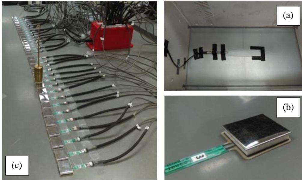
**Figure 7: Calibration setup of the (a) RPC and FSR: (b) modification of the sensor and (c) dead load used for calibration**
