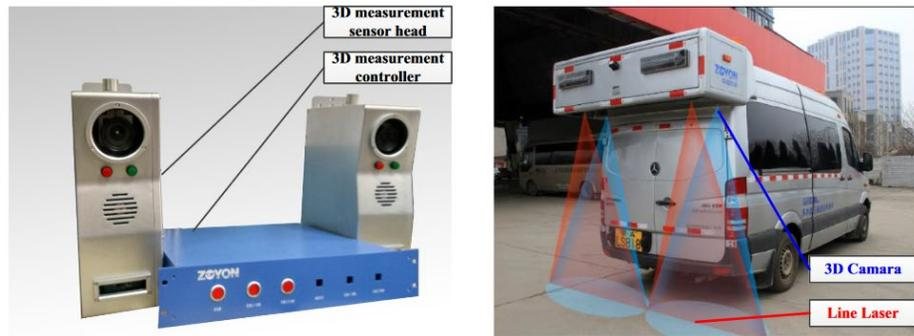
Figure 9. 3D-based Collection Measurement System
