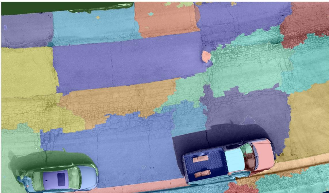
**Figure 31. Watershed-based Segmentation Sample Result**
