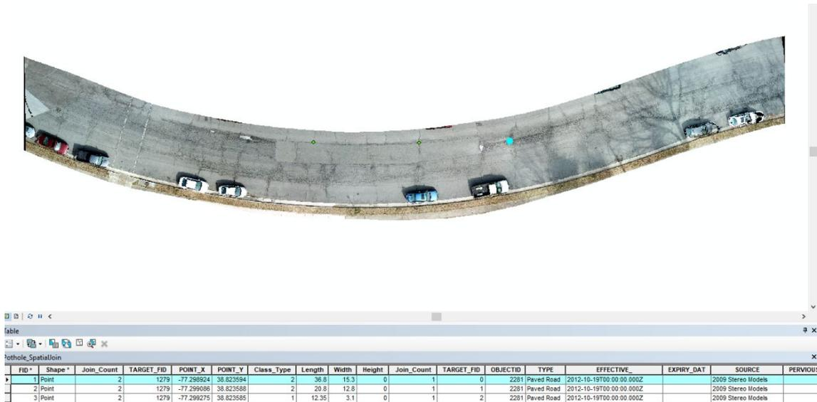
Figure 37. Tapestry Drive: Clipped Road and Pothole Data
