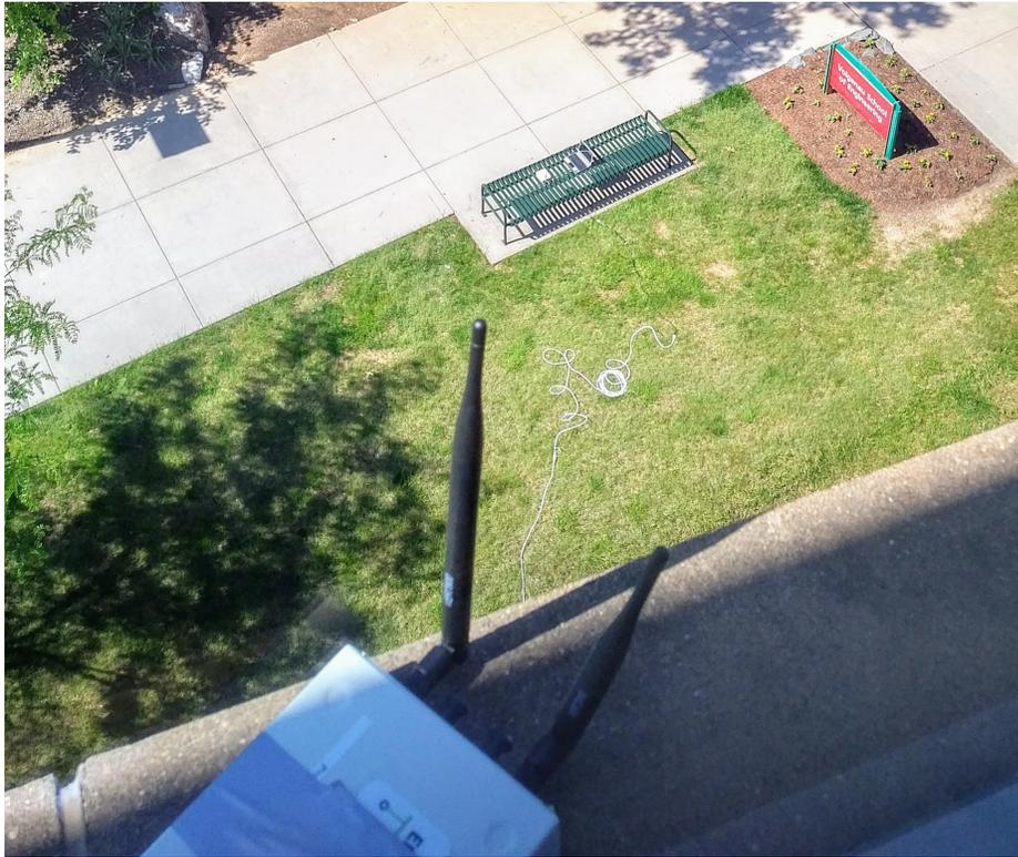
Figure 6.16: Test area that was used for elevation tests. Receiver is placed on the ground and the sender is elevated.
