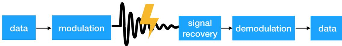
Figure 6.2: Steps of signal decoding
