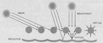
Since the tubes are round instead of flat, they can efficiently collect the sun's energy from any direction, just as if they were physically tracking the sun's path. And reflectors help collect the energy that does not fall directly on the tubes.
