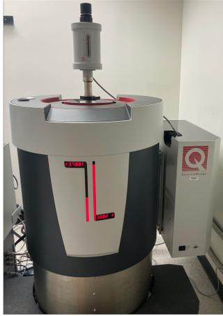
Figure B.4: Quantum Design Dynacool Physical Property Measurement System (PPMS) with a 9 T magnet. The DC magnetization (DCM) linear motor is shown by the small cylinder placed on top of the PPMS. Below is the chamber where the sample is located at the end of a long rod where high magnetic fields (up to 9 T) and low temperatures (down to 1.8 K) can be achieved.
