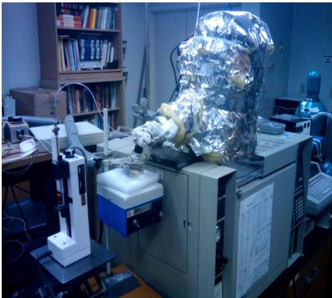
**Figure 5.** Photograph shows the experimental setup of the HSGC. The valves are inside the valve box insulated with fiberglass and aluminum foil. The thermostated sample cell is placed on the magnetic stirrer and the autosyringe next to it.
