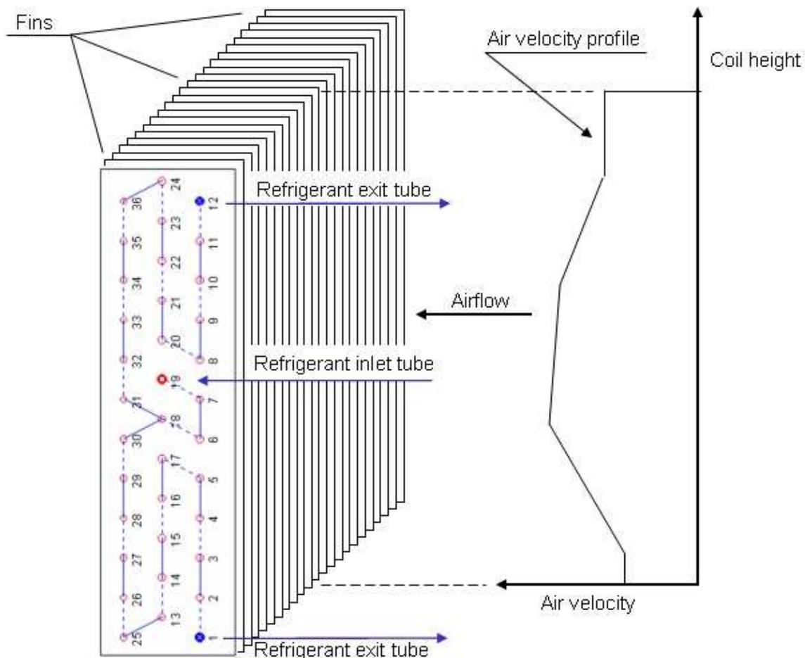
Figure 1. EVAP's representation of an evaporator
