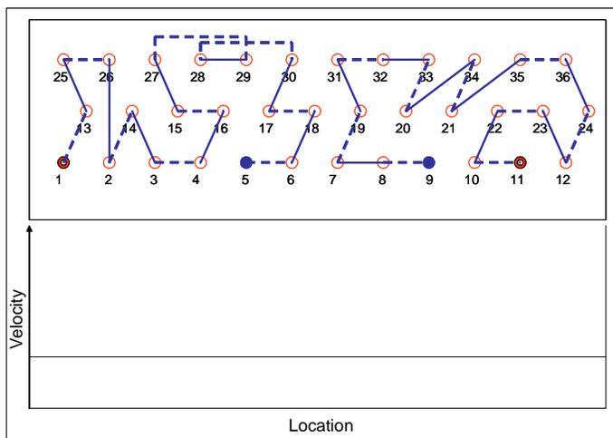
*Figure 4.* ISHED1-generated refrigerant circuitry for uniform air distribution:
