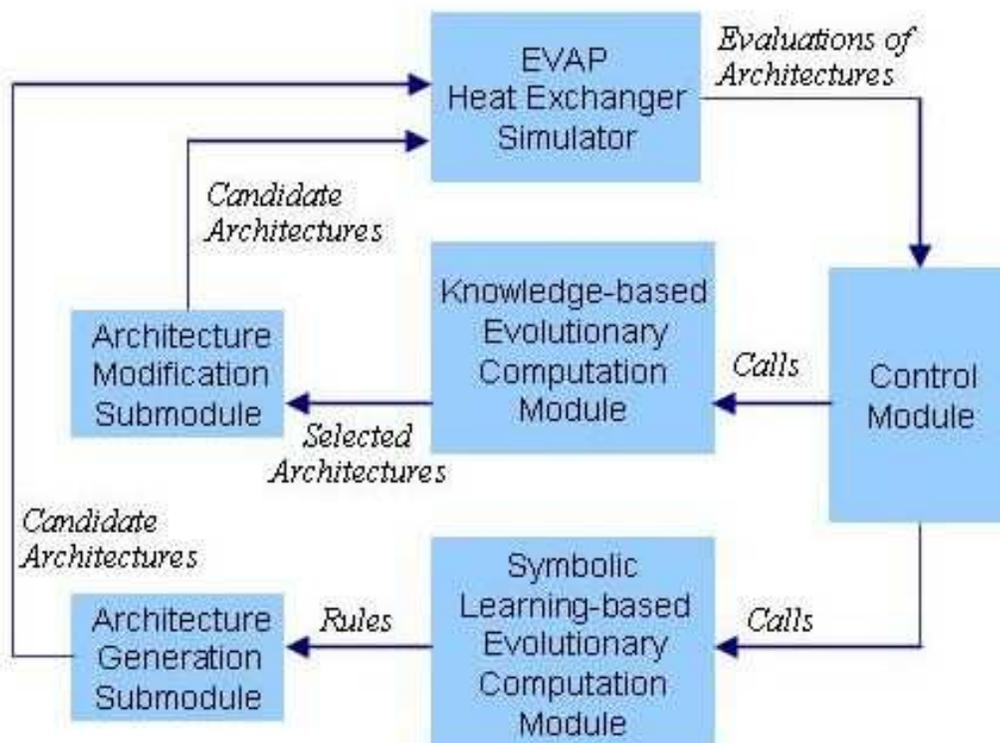
Figure 2. A functional architecture of ISHED1.
