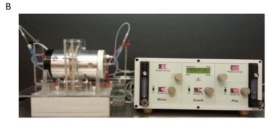
**Figure 1: Nanoaerosol Generator** (A) Schematic of the electrospray neutralization chamber and (B) photo of nanoaerosol generator with the electrospray neutralization chamber on top of the high voltage power supply (on left) and the electronic control panel (right).
