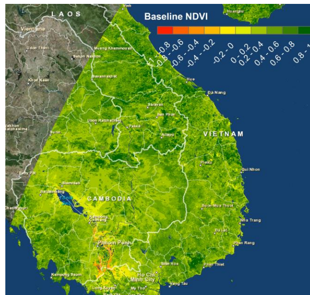
Figure 15 August NDVI: Note the area to the east of the Tonle Sap Lake appears slightly fuzzy or smeared. This is due to haze and thin clouds that are not fully masked. Future updates to the compositing system will incorporate the MOD35 Cloud mask.
