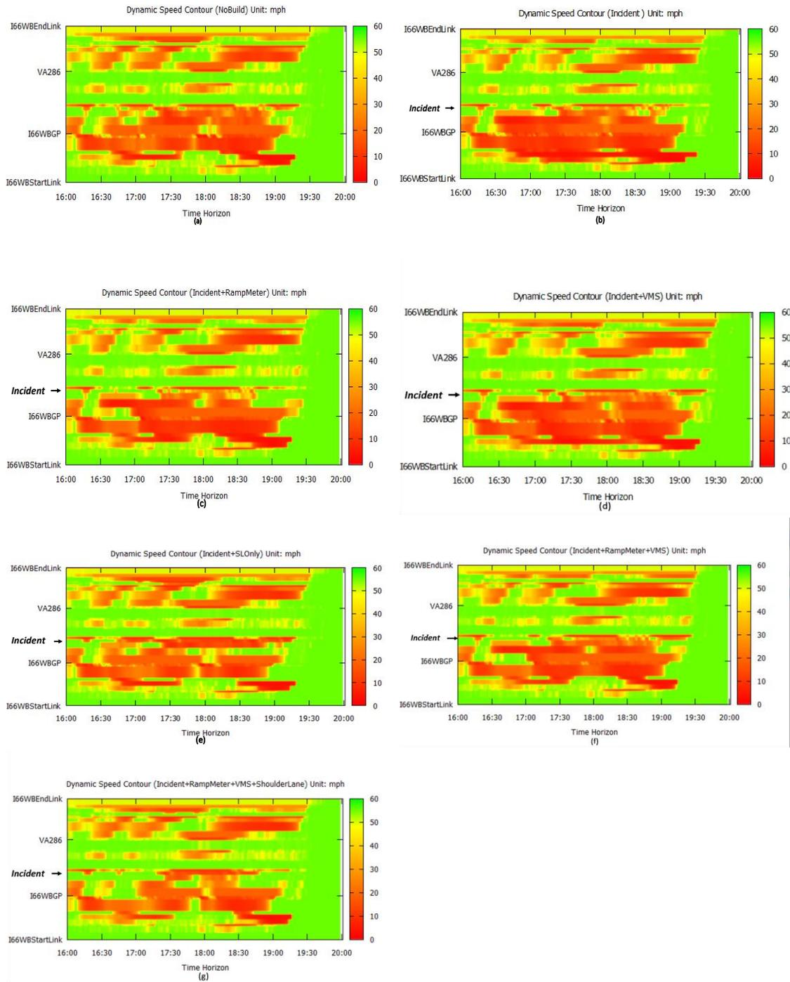
Figure 20. Corridor Travel Speed Heat-map under Different Incident and Control Scenarios
