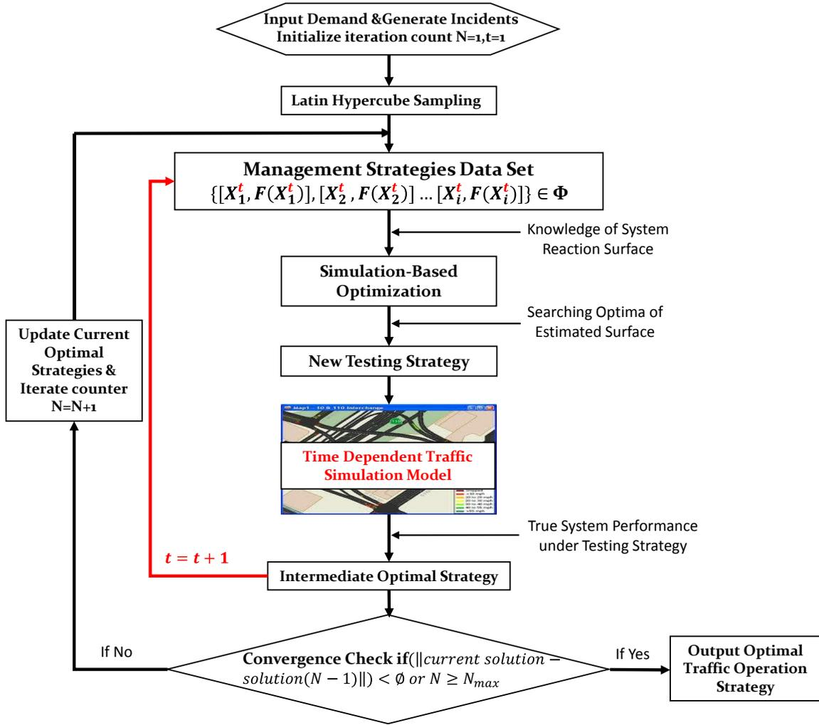
Figure 8. Framework of the Incident Response Optimization Model (Adapted from Chapter Three, New Components Highlighted in Red)
