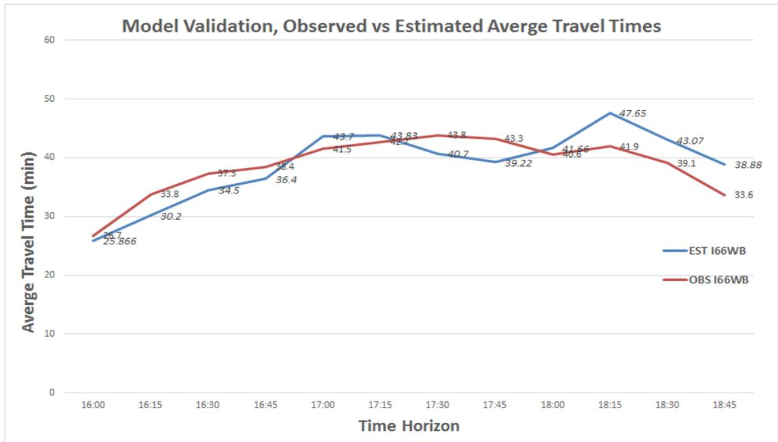
Figure 12. Observed vs. Estimated Corridor Travel Time on I-66WB
