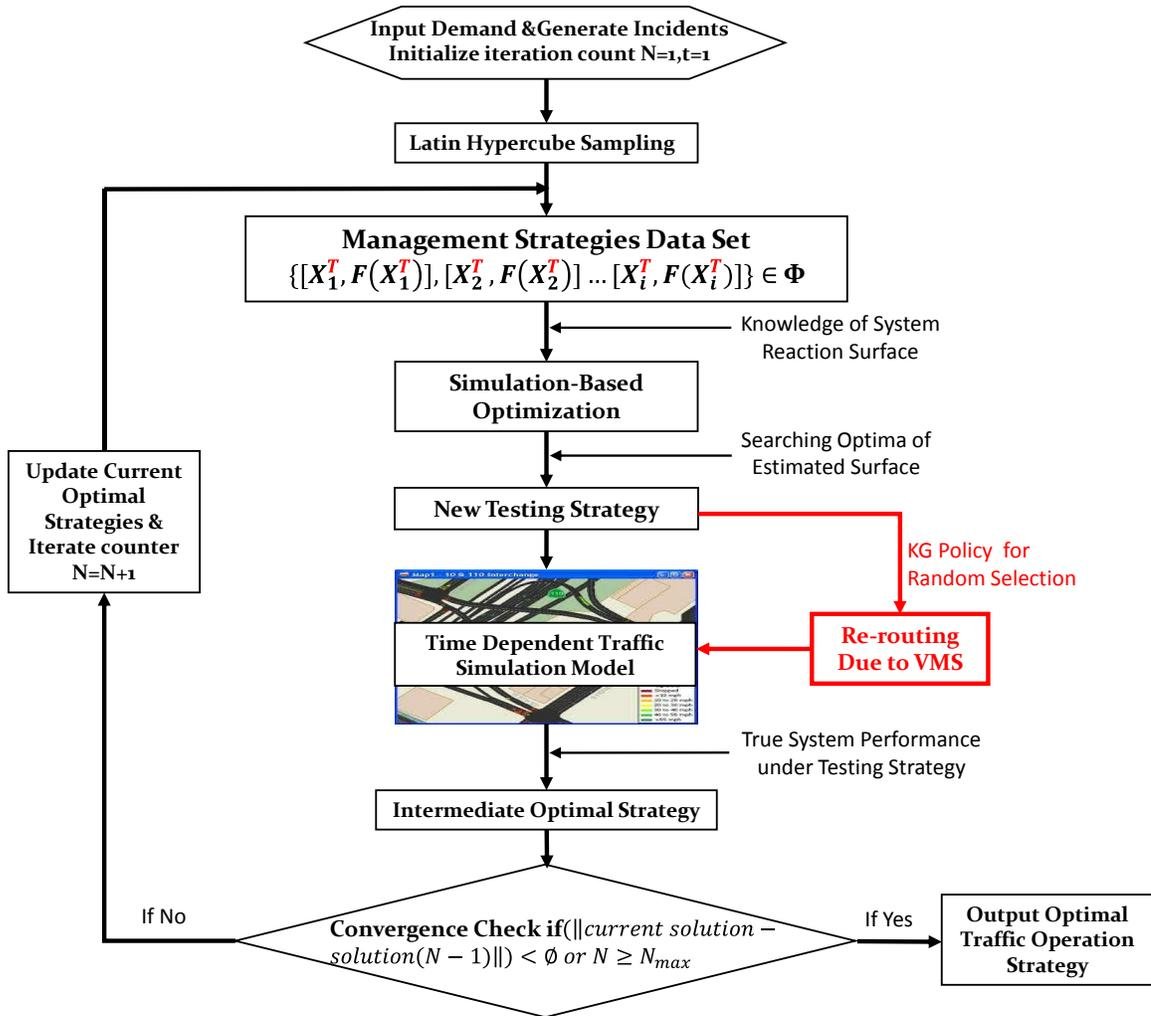
Figure 16. Framework of the Incident Response Optimization Model (Adapted from Chapter Four, New Components Highlighted in Red).
