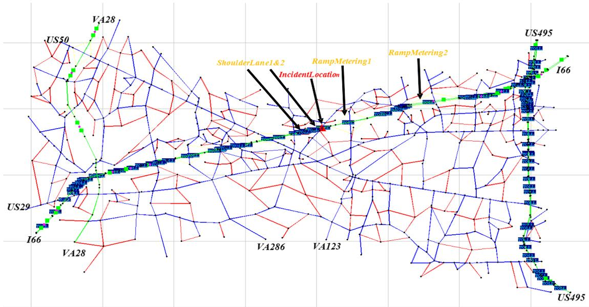
Figure 10. Simulation Network in DTALite
