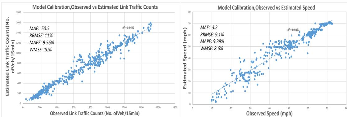
**Figure 11. Comparison between Observed and Estimated Link Counts and Speed**
