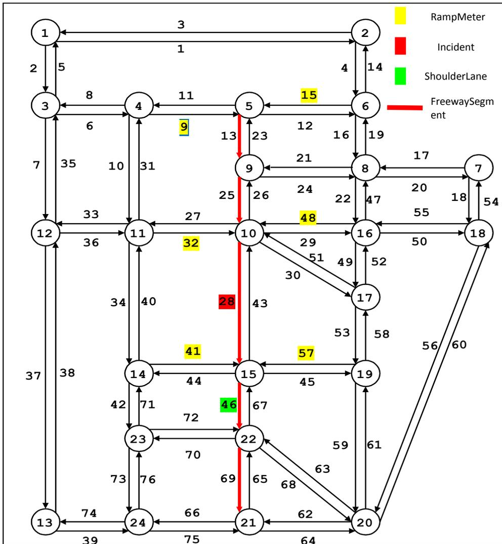
Figure 3. Sioux Falls Traffic Assignment Network.
