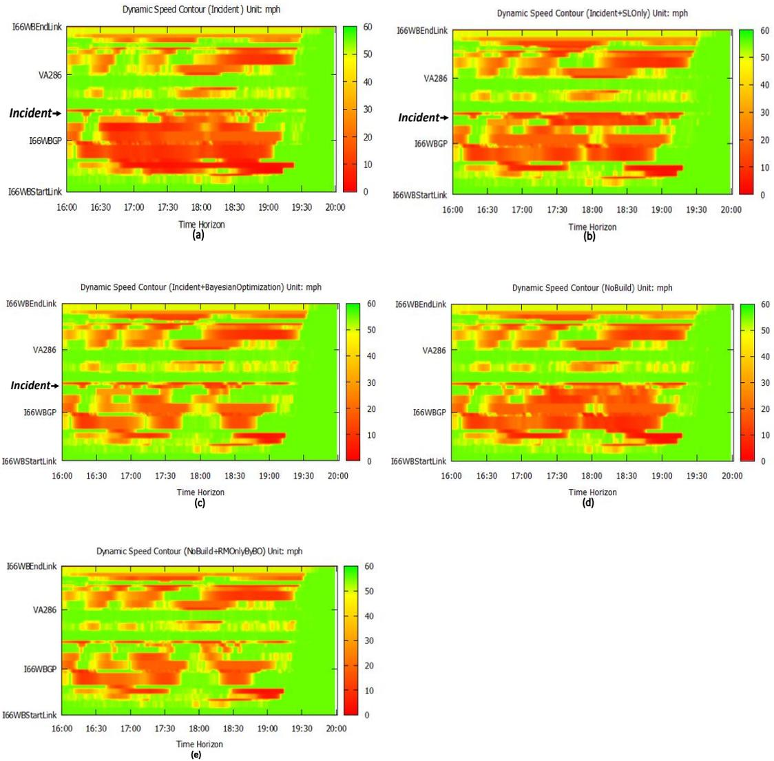
Figure 15. Corridor Travel Speed Heat-map under Different Incident and Control Scenarios
