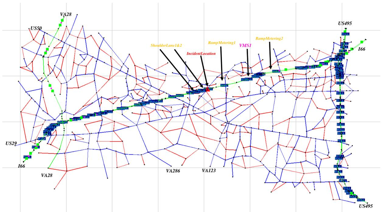
Figure 17. Simulation Network in DTALite with Multiple Traffic Operation Controls
