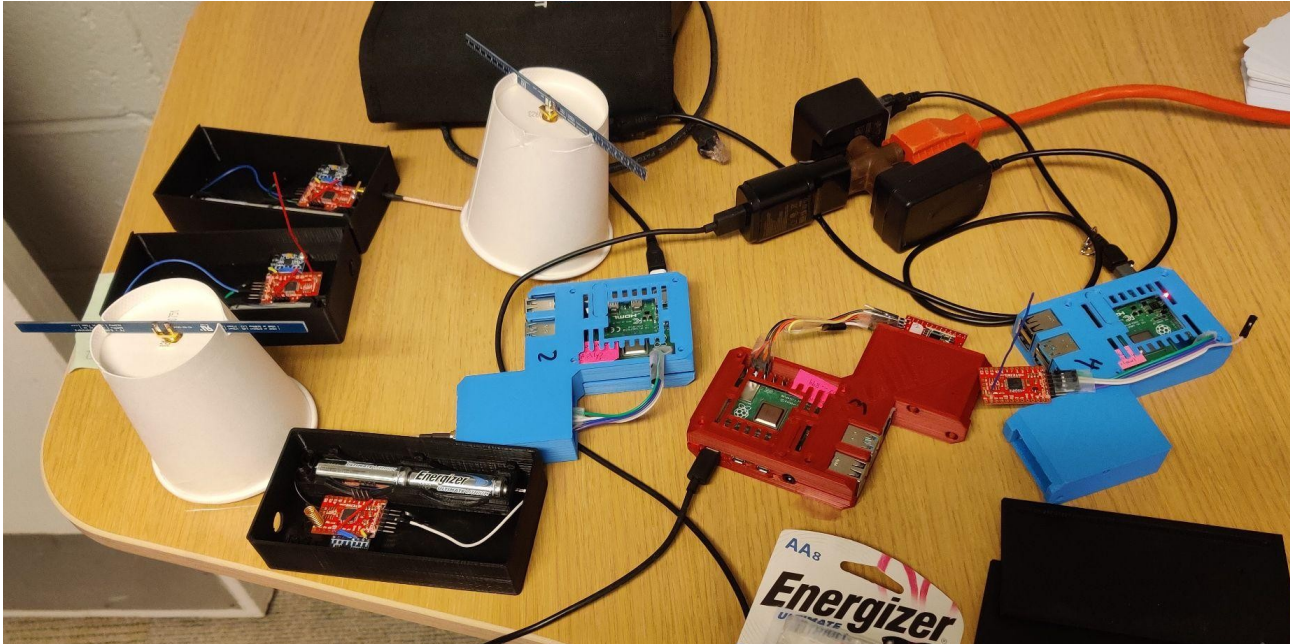
Figure 9. Base stations and transmitter units used for transceiver validation
