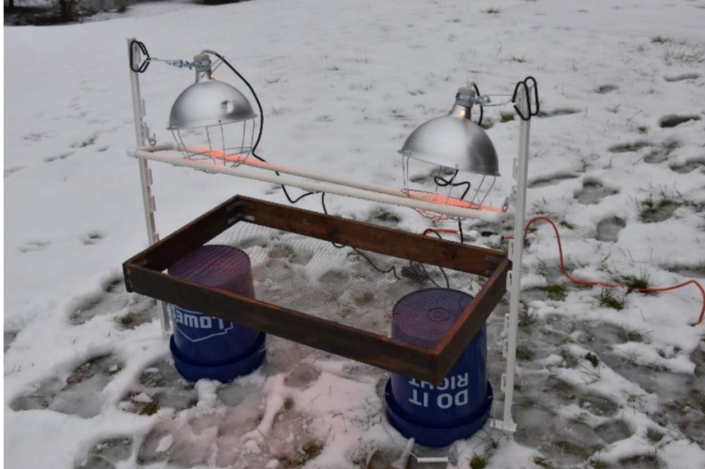
Figure 7. Sifter setup under heat lamps
