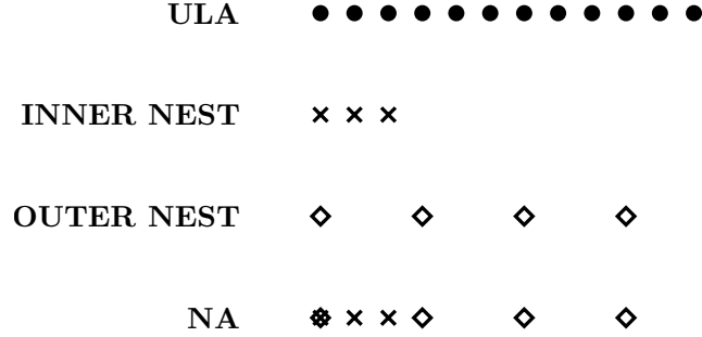
Figure 2.12: Array geometry for a 12 sensor ULA and 6 sensor NA with the inner nest using Q = 3 sensors with d m spacing and the outer nest with P = 4 sensors and 3d m spacing. The first element is common to both subarrays.
