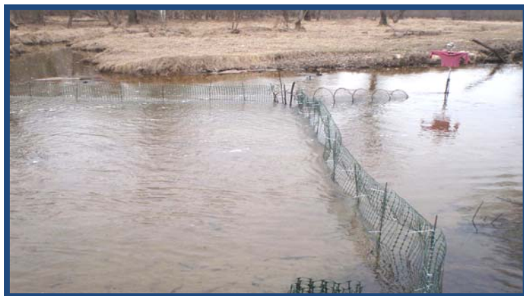
Picture 1. Hoop net deployed in Pohick creek. The top of the hoop net is exposed at both high and low tide to avoid drowning turtles, otters, or other air-breathing vertebrates. The hedging is angled downstream in order to funnel up-migrating herring into the opening of the net. The scarecrow was used to deter river otters from entering the net.
