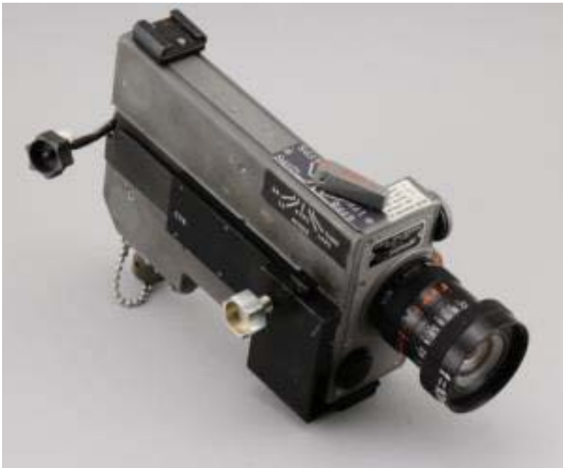
Figure 57 - Data Acquisition Camera from the Apollo 11 Lunar Module, NASM Cat. # T20140016083 (NASM Photo).
