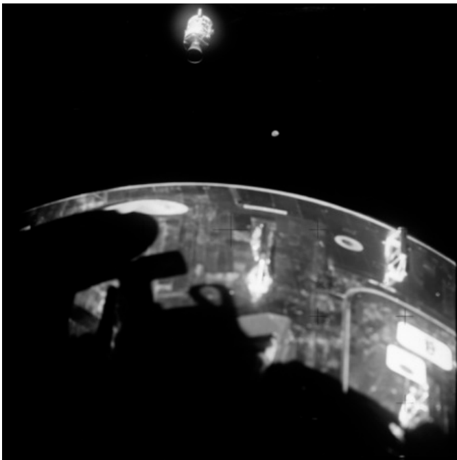
Figure 59 - Magnification of the Service Module in the upper portion of the photograph gave engineers their only look at the damage to Apollo 13, April 17, 1970, AS13-59-8500 (NASA Photo).
