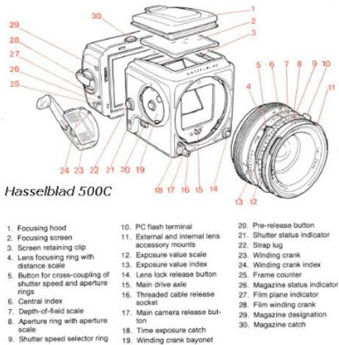
Figure 47 - Diagram of Hasselblad 500c model and its parts (Hasselblad 500C Instruction Manual).
