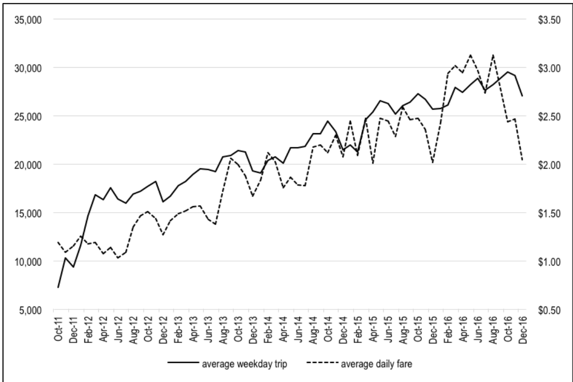
Figure 6 I-85 Express Lanes average weekday trips and fare, Oct 2011 – December 2016 (State Road and Tolling Authority 2017b)
