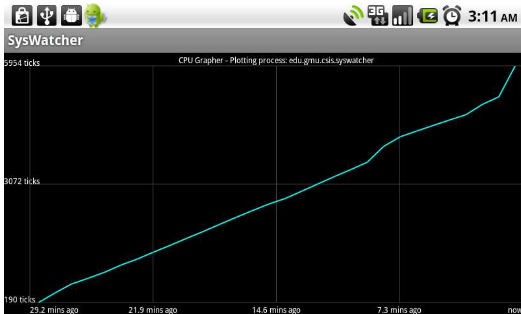
Figure 5.3: Metering process CPU utilization graph.
