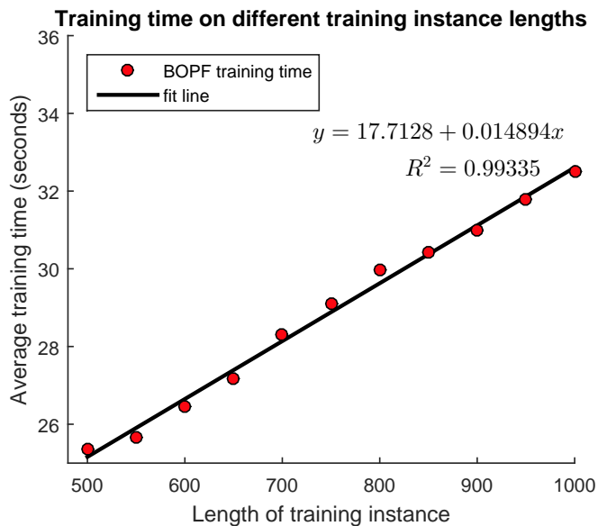
Figure 2.5: Training time of BOPF on different training instance lengths.
