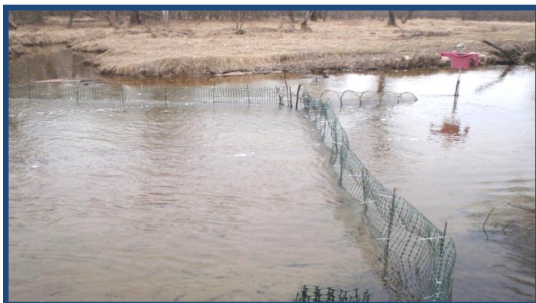
Figure 1. Hoop net deployed in Pohick creek. The top of the hoop net is exposed at both high and low tide to avoid drowning turtles, otters, or other air-breathing vertebrates. The hedging is angled downstream in order to funnel up-migrating herring into the opening of the net.
